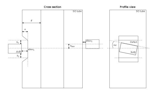
**Figure 7.1** – Geometrical parameters of the computer model C3D. Left: Profile view of a steam generator tube where the left AVB caused wear. Right: View of the side with the defect.
