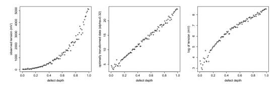
**Figure 7.2** – Left: Measured tension as a mapping of defect depth for 100 defective tubes. The other "nuisance" geometrical parameters are representative of possible geometries. Right: Same data after applying the logarithm function ( $B_{\alpha}$  or  $C_{\alpha}$  with  $\alpha = 0$ ) to all measured tensions. Center: Same data after applying the optimal transformation ( $C_{\alpha}$  with  $\alpha = 0.32$ ) to all measured tensions.
