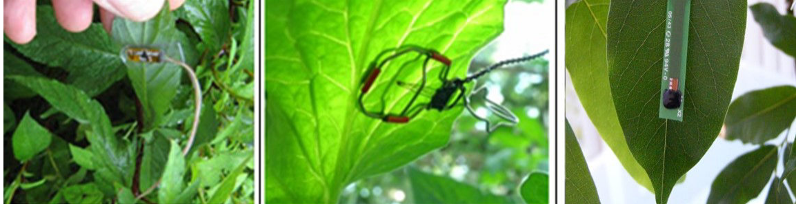
(A) SG-1000 leaf sensor by Agri-biotech company agriHouse, inc to monitor water deficit in plant[39].
