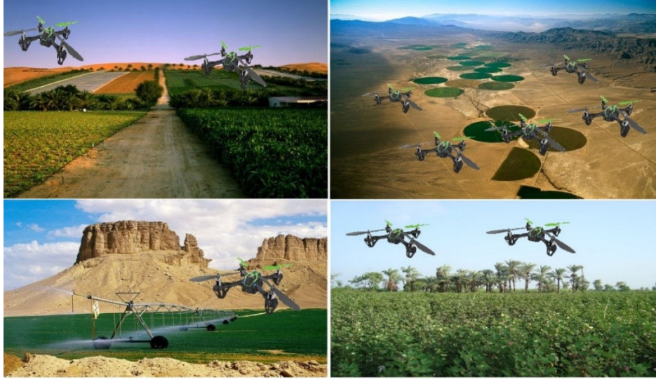
A set of UAVs can scan all/selective gateway nodes in all circular/rectangle farm fields by taking a flight over predefined way. These UAVs may have equipped with receiving devices, cameras, Navigation/GPS system.
