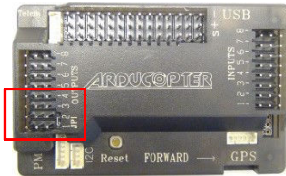
Figure 5.5: Arduino output pins for ESCs
