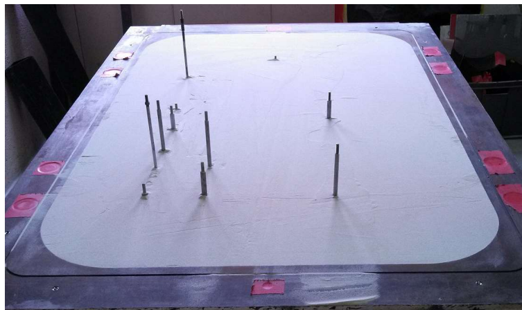
Figure 26. Sand sample reconstituted with helical anchor models placed during pluviation.
