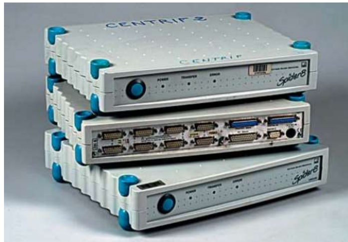
Figure 124. Spider data acquisition modules (Thorel, et al., 2009).
