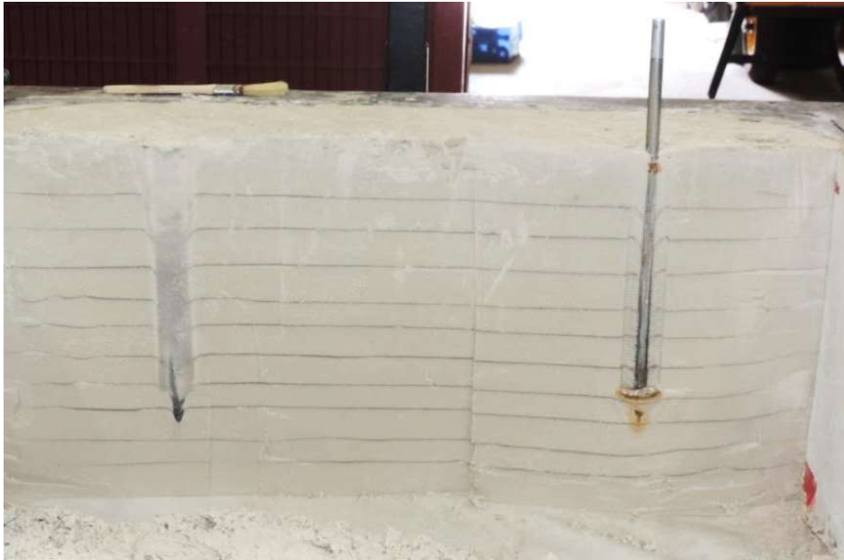
Figure 28. Sample excavation for the visualisation of installation and failure mechanisms.
