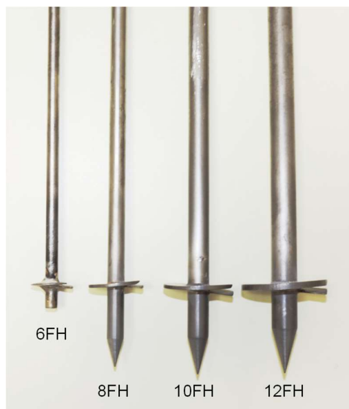
Figure 23. Helical model anchors with fixed helix.
