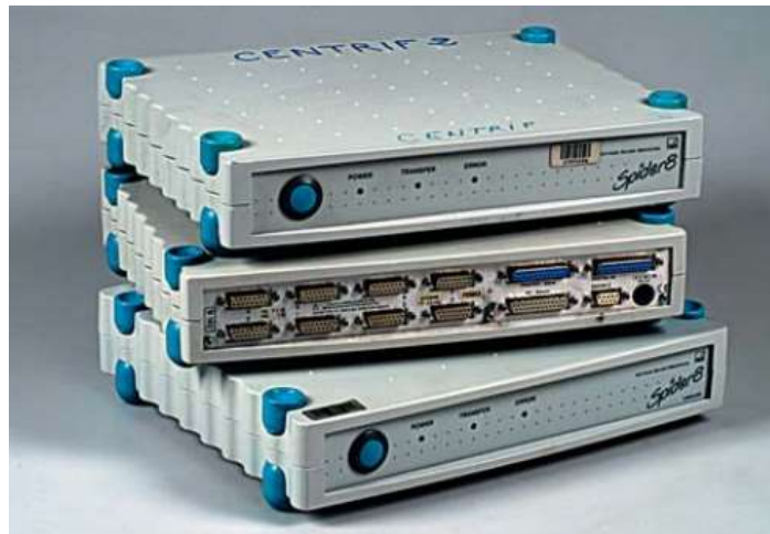
Figure 124. Spider data acquisition modules (Thorel, et al., 2009).
