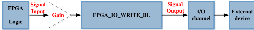
Fig.5.16 Signal flow diagram from FPGA of MicroLabBox to external device
