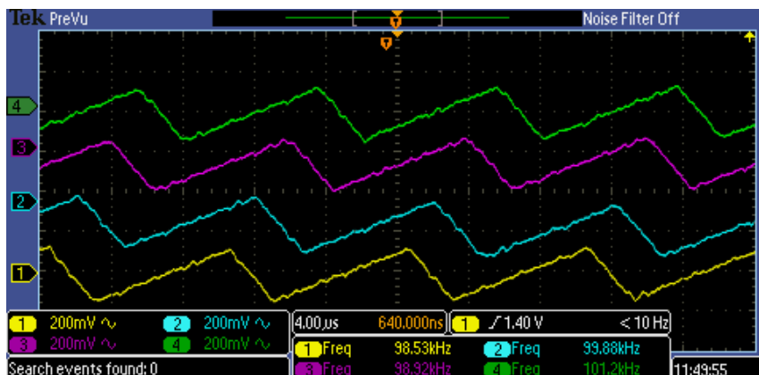
(h) AC component of I_{L1} (yellow, 200mV/div is equivalent to 2.2A/div), I_{L2} (blue, 200mV/div is equivalent to 2.2A/div), I_{L3} (purple, 200mV/div is equivalent to 2.2A/div), and I_{L4} (green, 200mV/div is equivalent to 2.2A/div) signals' frequencies.
