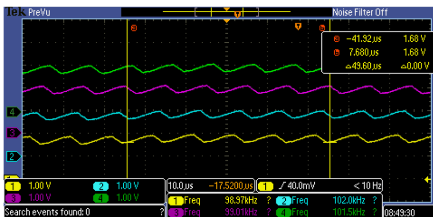
(h) I_{L1} (yellow, 1.00V/div is equivalent to 11A/div), I_{L2} (blue, 1.00V/div is equivalent to 11A/div), I_{L3} (purple, 1.00V/div is equivalent to 11A/div), and I_{L4} (green, 1.00V/div is equivalent to 11A/div) signals' frequencies.
