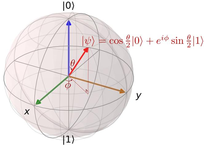
Figure 1.1: The Bloch sphere with antipodal points corresponding to a pair of mutually orthogonal qubit states. The north and south poles of the Bloch sphere are chosen to be  $|0\rangle$  and  $|1\rangle$ . The points on the surface of the sphere correspond to the pure states of the qubit, whereas the interior points correspond to the mixed states.
