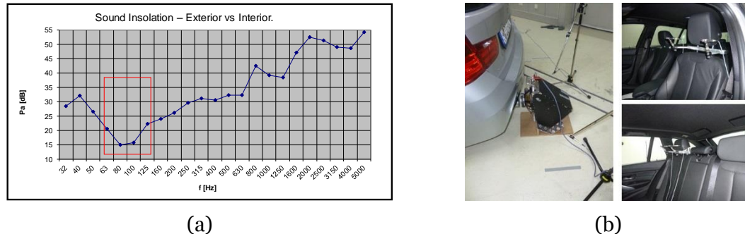
Figure 1.3: (a): Sound insulation in 3 rd octave representation. A minimum is observed in low frequency range—marked with the red rectangle. This critical insulation could result in exhaust-inferred booming; (b): Measurement setup showing the external acoustic source and the microphones’ positions inside the car.
