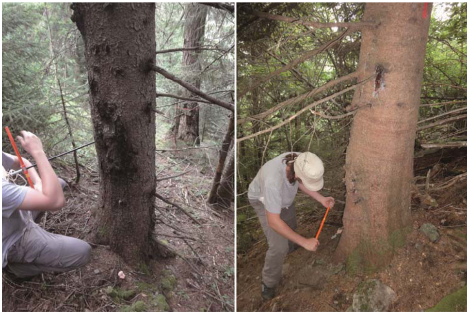
Figure 8. Increment borer used in forestry to extract cores.
