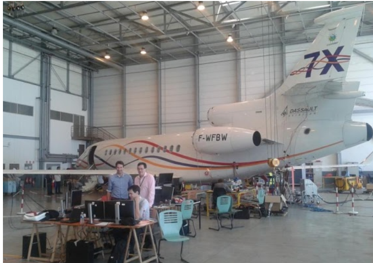
Figure 6.2: Falcon 7X s/n 001 during ground vibration test (with some Dassault-Aviation colleagues).
