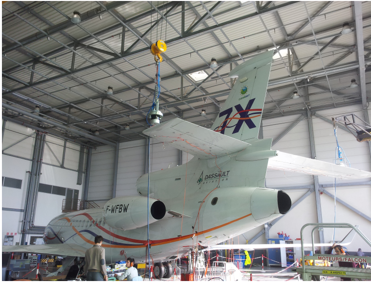
Figure 2.12: Left: Ground vibration experimental test-bed. Right: illustration of the sensors location.
