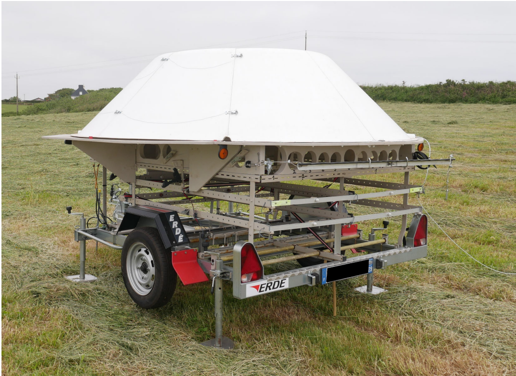
Figure A.3.: The SODAR (SONic and Detection And Ranging) device used fo the onshore kite measurements. Source: Behrel et al. (2017)
