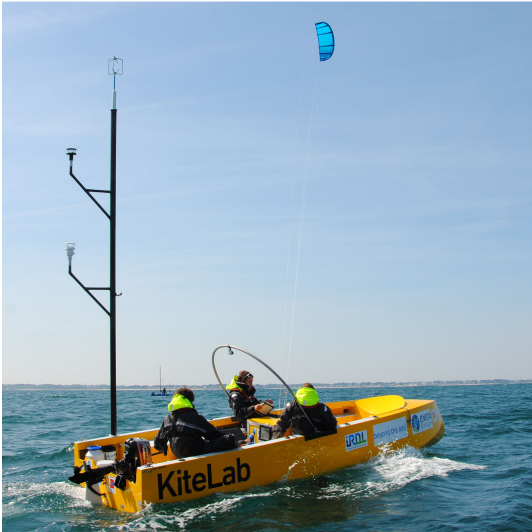
Figure A.1.: Picture of the KiteLab, the experimental platform specifically designed to carry out measurements on effects and performances of kite propulsion. The 5-meter wind measurement mast is visible on the rear of the boat. The inflatable kite flying over the boat is a 5 m 2 one. Source: Behrel et al. (2017)
