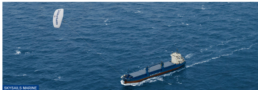
Figure 1.2.: A Skysails kite of 320 m 2 on a 90 m long cargo ship
