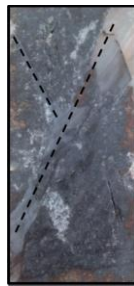
(m) sample with two faults after experiment
