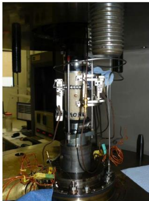
Figure 5.2 Sample assembly on tri-axial cell at GFZ Potsdam, Germany (Reinsch et al., 2012)
