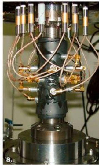
Figure 1.2 Ultrasonic sensors and strain gauges glued on samples (from Ougier-Simonin et al., 2010, 2011)
