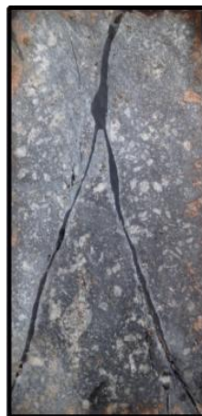
(i) Sample after experiment with a fork shaped fracture
