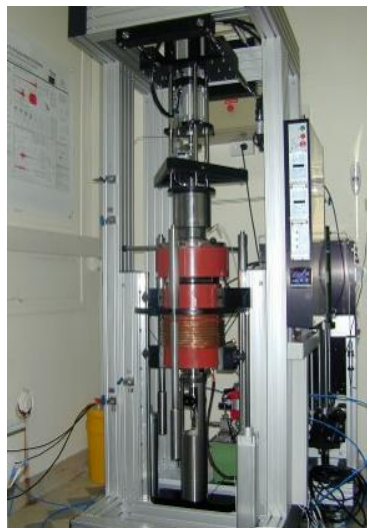
Figure 1.1 Tri-axial cell installed at École Normale Supérieure (Ougier-simonin et al., 2010, 2011)
