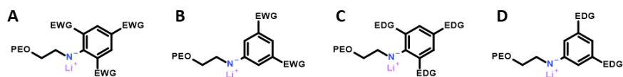
Illustration 1 – Hypothetical end-group designs based on an N -aryl secondary amine. The aryl ring is modified with Electron Withdrawing Groups (EWGs), and Electron Donating Groups (EDGs). A phenyl ring is illustrated for simplicity.
