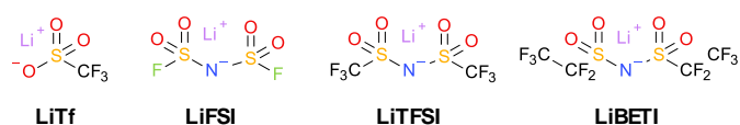
Figure I-5: The fluorinated sulfonate lithium salt (LiTf), and the sulfonylimide salts lithium salts (LiFSI, LiTFSI, and LiBETI)
