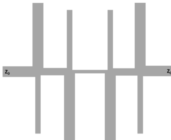
Figure I.20 : Filtre DBR "Dual Behavior Resonator".
