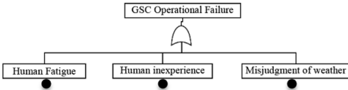
Fig. 3.7 FTA of the GSC operational failure: the GSC operational failure is one of the cause of communication failure. GCS, which is controlled by human, can have degradation in the performance due to human fatigue, inexperience or due to a misjudgment of the weather.
