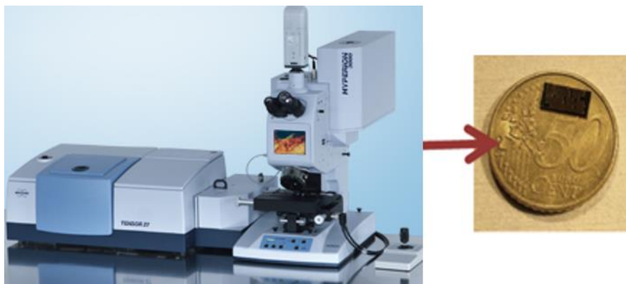
Fig.5.1.3. Comparison of conventional bulky Fourier-Transform spectroscopic system and on-chip integrated system.
