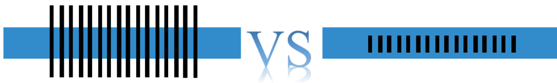
Fig.3.2.9. Schematic top view of the optical mask of waveguide Bragg grating, (left) first design, (right) optimized design.
