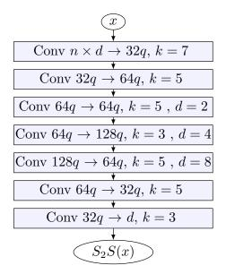
Figure 4.6: Architecture for S2S-dil model, taking the segmentations of n=4 frames in input, each of channel dimension C. Each inner convolutional layer is followed by a ReLU. Each convolutional layer has a kernel of size  $k \times k$  and dilation parameter d. q is a hyperparameter used to scale the number of feature maps linearly for simple control over the model capacity. Stride is always one and padding is chosen so as to maintain the size of the input.
