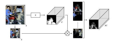
Figure 3.3: Illustration of using the product of the RGB input and the output of the segmentation network to generate input for the discriminator. The image is down-sampled by the stride of the segmentation network. The probability maps are then multiplied element-wise with each colour channel. These outputs are concatenated and form the input to the discriminator.
