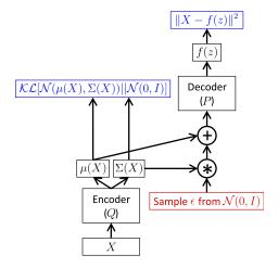
Figure 2.7: Training a VAE involves jointly training an encoder and a decoder. Red blocks are non-differentiable sampling operations. Blue blocks represent loss terms. Figure adapted from (Doersch, 2016).
