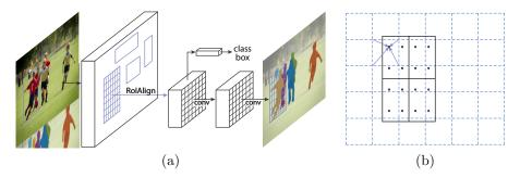
Figure 2.4: (a) The Mask R-CNN framework for instance segmentation. (b) RoIAlign: The dashed grid represents a feature map, the solid lines an RoI (with  $2\times2$  bins in this example), and the dots the 4 sampling points in each bin. The value of each sampling point is computed by bilinear interpolation from the nearby grid points on the feature map. Both figures from (He et al., 2017).
