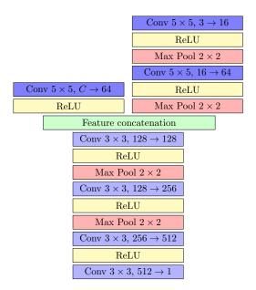
Figure 3.2: Discriminator architecture used for the Stanford Background dataset. The left and right branch processes respectively the class segmentations and the RGB image.
