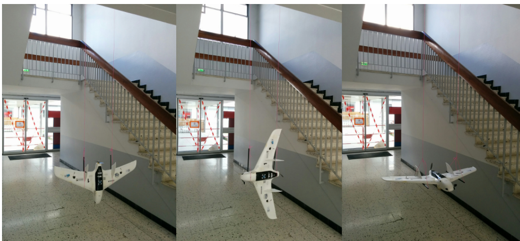
Figure 3-7: Moments of inertia measurements for each axis, I_{xx} , I_{yy} , I_{zz} .
