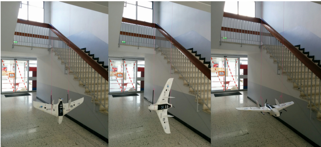
Figure 3-7: Moments of inertia measurements for each axis, I_{xx} , I_{yy} , I_{zz} .
