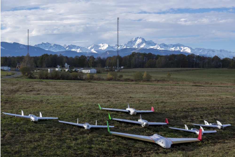
Figure 2-5: Fleet of Paparazzi equipped drones from ENAC UAV laboratory in a flight campaign with the Pyrenees in the background. Photo by Alexandre Bustico.
