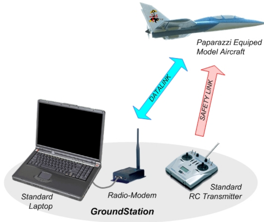
Figure 2-6: Paparazzi Autopilot System overview
