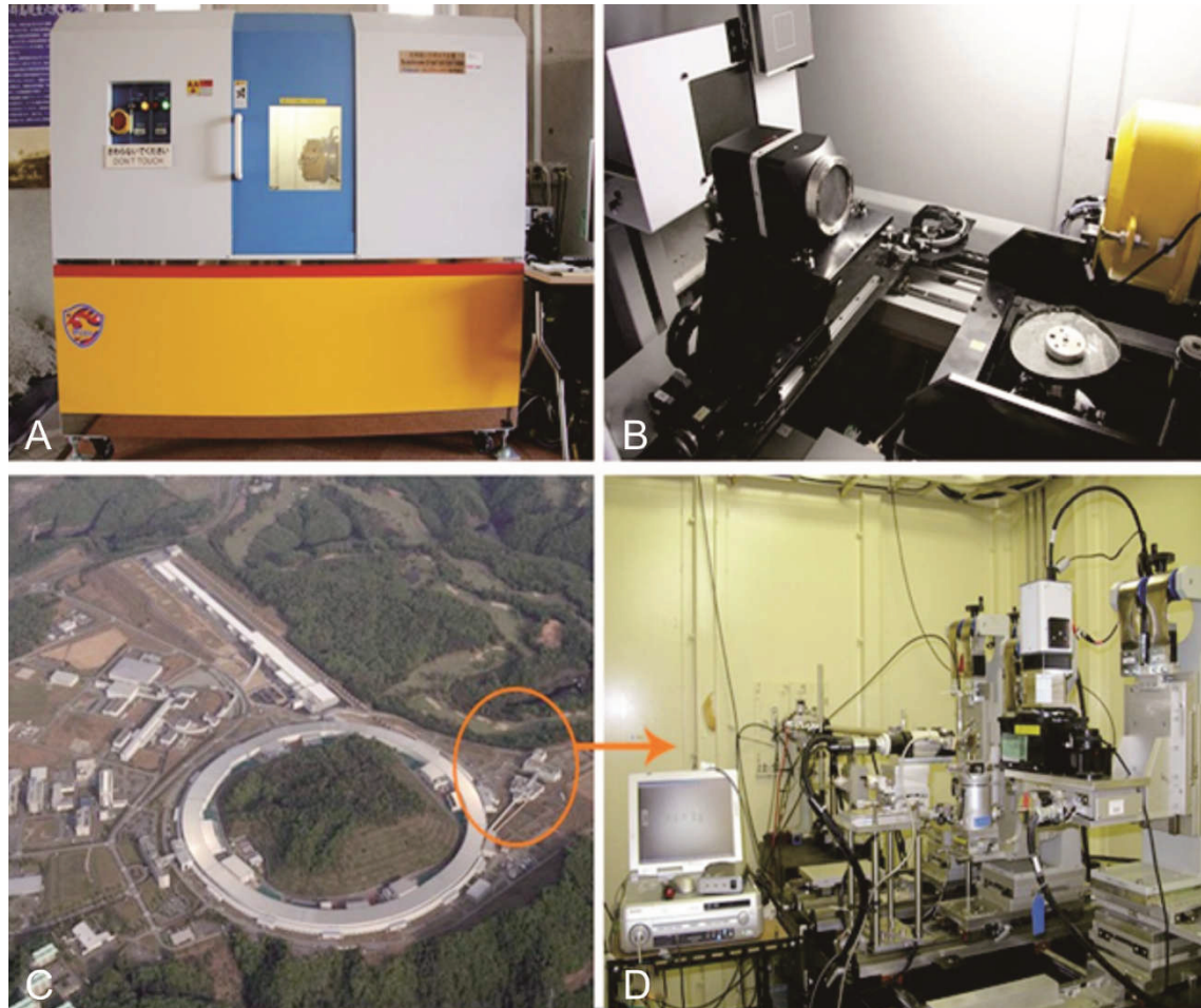
Fig. 68. A-B. The computed X-ray Microtomography (XTM) at Tohoku University, Japan. C-D. The synchrotron X-ray Microtomography (SRXTM) at Spring-8 in Hyogo, Japan.
