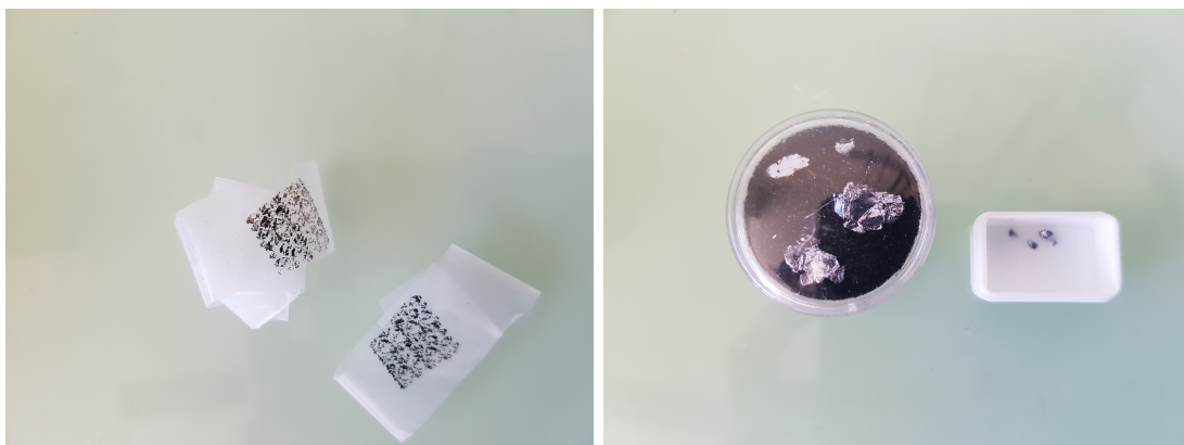
Figure 3.10 – (left) Picture of exfoliation on scotch tape executed by the above explained method using (right) natural and HP/HT crystal of MoS 2 .
