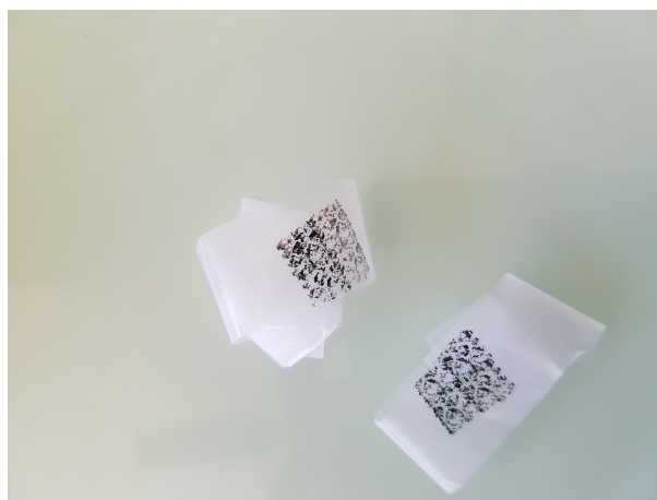
Figure 2.5 – Homogeneous square-like structure of flakes obtained after repeated exfoliation steps on the same scotch tape
