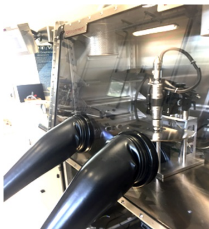
Figure 5.34 – Picture of microtransfer machine built inside the glove box with Argon atmosphere.
