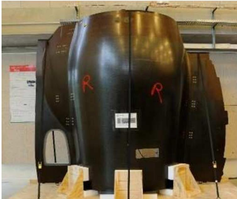
Figure 1.2 – Aircraft nacelle’s Inner Fixed Structure.
