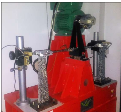
Figure 24 - Essai de fatigue.
