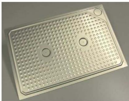
Figure 0-39: CSM panel containing PCM [102]
