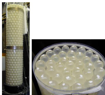
Figure 0-14: cylindrical LHES filled with PCM spheres [48]
