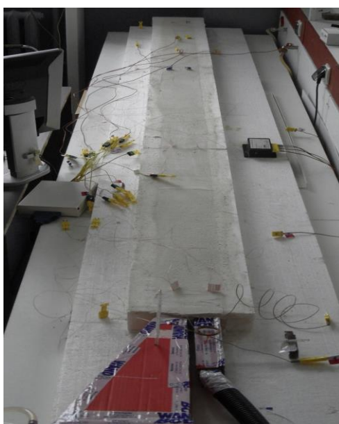
Figure 0-50: ceiling panel made of gypsum-PCM composite [123]
