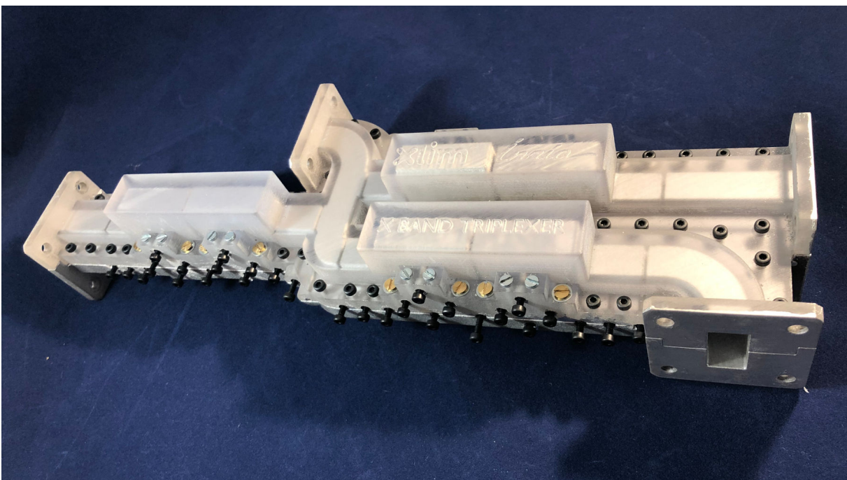
Figure E.10: Triplexer final structure: front view.
