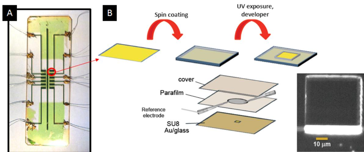
**Figure 2.4:** (A) Photo of the 12-electrode ensemble after the lithographic process. (B) Sketches of the microfluidic cell preparation. The inset shows a dark field image of the electrode surface - the square consists in exposed Au, while all the surroundings are recovered by a  $Si_2N_3$  insulating layer.
