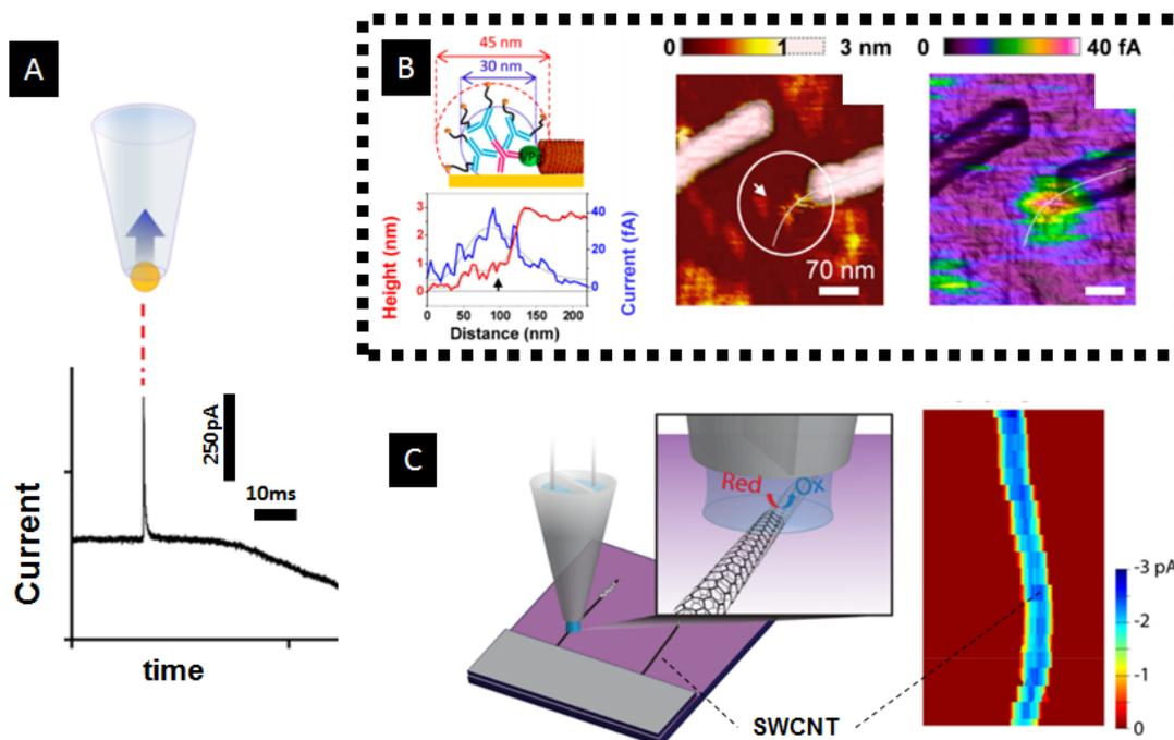
**Figure 1.6:** Electrochemical methods for studying individual objects (A) Nanopipettes as Coulter Counter: the passage of one particle modifies the conductivity of a nanopore leading to a peak, which can be used to size the nanoparticle (Adapted from [50]). (B) AFM-SECM coupled approach for studying the distribution of redox active groups over a single virus (Adapted from [56]) (C) SECCM image of the reactivity of a Single Walled carbon nano wire (Adapted from [62]).
