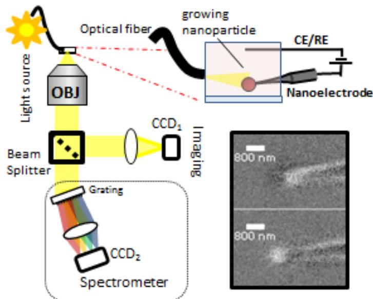
**Figure 4.2:** Dark Field Setup for nanoparticle monitoring over an electrode. The inset shows an example of cathodic particle growth: the application of a 5s -1V pulse leads to the appearance of a small particle (smaller than the point spread function). Both images have been subtracted of an image taken just before the application of the pulse.
