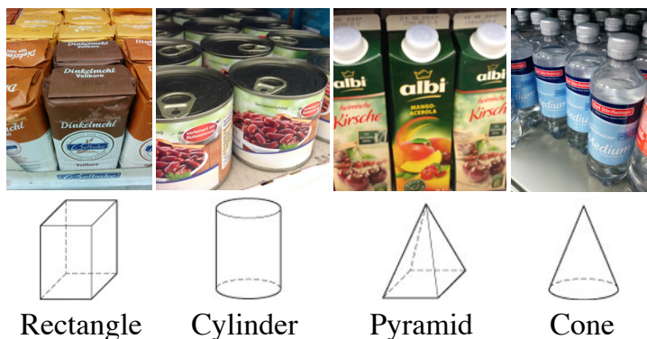
Figure 6.2: Main product shape categories, that comprise 90.1% of items in the dataset, are defined based on the the shape of their base and their tip. The shape of the tip determines whether the objects can be stacked or not. The shape of the base determines whether the object is more compactly arranged on a regular grid (rectangular) or an off-grid arrangement (circular).
