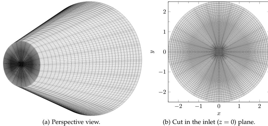
Figure 4.15: Mesh used for 3D nonlinear computation.
