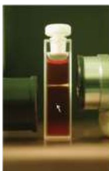
Figure 1.16 Illumination with one-photon (upper beam, 532 nm) and two-photon wavelengths (lower beam, 1057 nm) [28]
