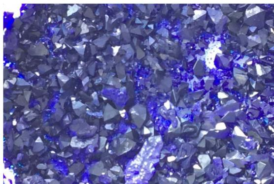
Figure 151: Picture of crystals obtained after synthesis with average size around 0.5  $\mu\text{m}$
