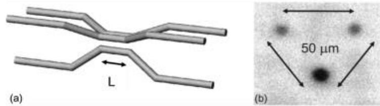
Figure II.14: (a) Schematic presentation of the 3D coupler (b) Mode profiles of the output indicating that the light is coupled in the three branches with a ratio of 43%:28%:29%. Taken from [111].
