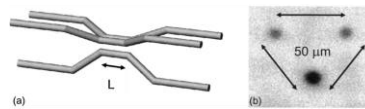
Figure II.15: (a) Schematic design of the 1 to 8 beam splitter with 7-Y junctions (b) Side view output of the far-field modes [113] .....57
