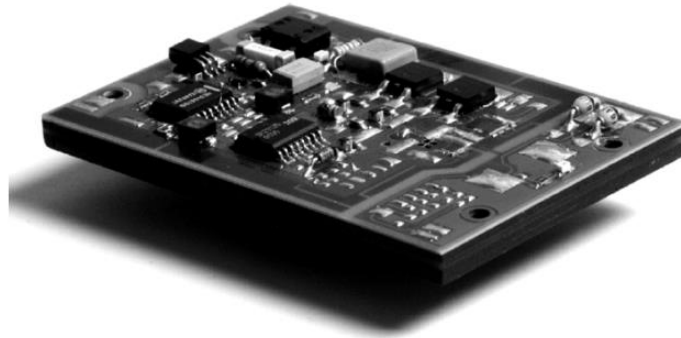
Fig.1-6. Thin 60-W offline converter with PCB integrated transformer and capacitors [40]
