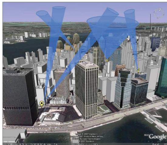
Figure 1.4. Example of NLOS UV communication, source: [15]
