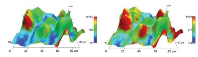
FIGURE 4. Total elastic (or deformation) work colored topography
