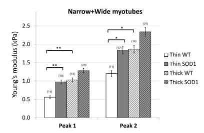
FIGURE 26. Average elasticity of wild-type and SOD1 mutant myotubes. The bars (Peak 1 and Peak 2) represent the mean of the double Gaussians, fitted on the elasticity value distributions of individual force maps. In brackets the number of the analyzed force maps is marked. Error bars are the standard error of the mean. As indicated, the elasticity of thin wild-type (WT) myotubes is significantly lower than thin SOD1 and thick wild-type as well (\* p < 0.05, \*\* p < 0.01).
