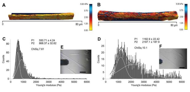
FIGURE 24. Elasticity color-coded 3D-reconstruction of representative thin (A) and thick (B) wild-type myotubes. Yellow color shows softer portions, while red to blue colors show stiffer regions. C and D are the elastic modulus distributions of the corresponding force maps, where light gray curves are single Gaussians, while black curves represent the sum of the two. Insets E and F are optical images about the measured myotubes. Scale bars are 30  $\mu$ m.
