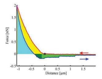
**FIGURE 2** A representative force-distance curve. Contact point is marked with "o," cyan area marks the plastic work, cyan + yellow area marks the total elastic work and sum of dark and light green area represents the total adhesion work
