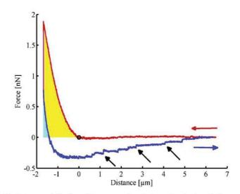
**Fig. 2.** A representative force-distance curve. Trace is drawn in red, retrace in blue. Contact point is marked with "o", cyan area marks the remanent work, cyan + yellow area marks the total work, black arrows indicate the place of located rupture events.
