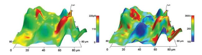
**FIGURE 6.** Maximal adhesion force colored topography
