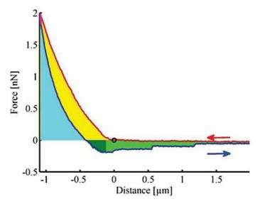
**FIGURE 2.** Representative force-distance curve collected along SCFS measurements. Contact point is marked with "o," cyan area marks the remnant work, yellow area marks the dissipated work, while the sum of dark and light green areas represent the total detachment work.
