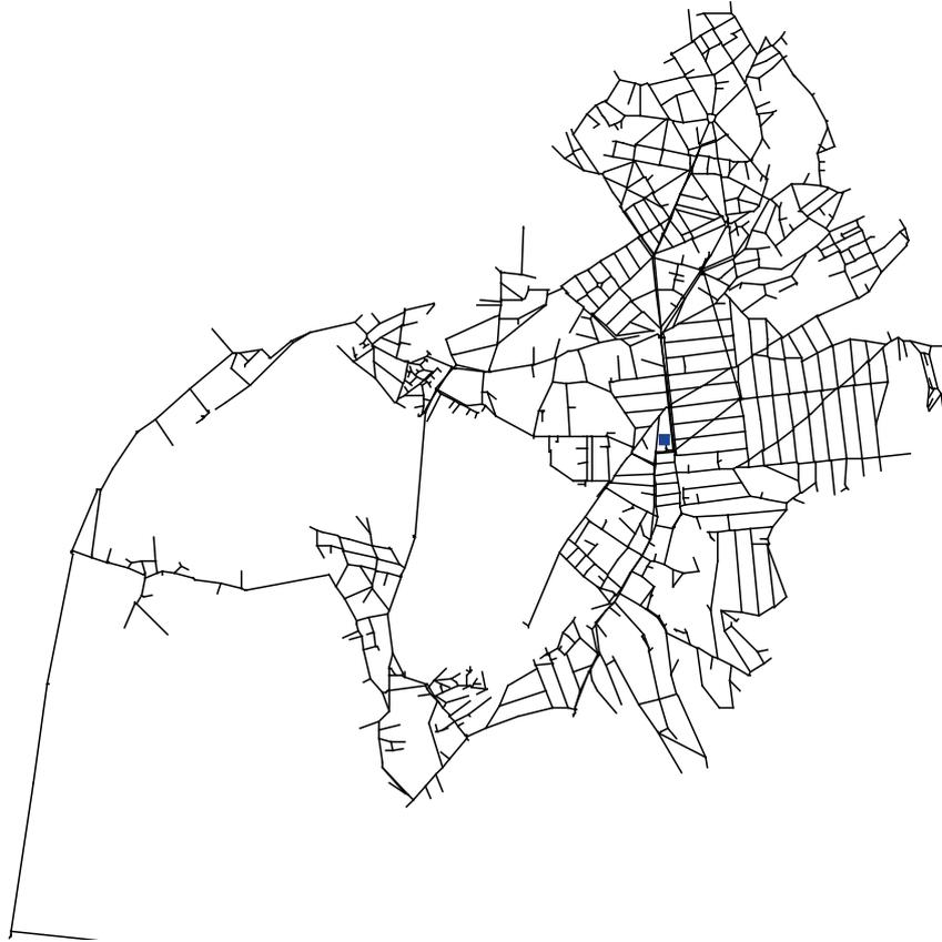
Figure 2.4: Realistic water distribution network from the Paris region, consists of a total number of 2,175 pipes, 1,822 nodes and one reservoir (indicated by the blue square).
