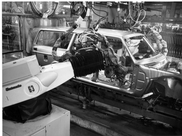
Figure 1.1: Unimate, invented by George Devol for General Motors in 1961 [Wallén 2008]
