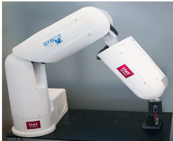
Figure B.1: Prototype of the 6-DOF ISYBOT collaborative robot
