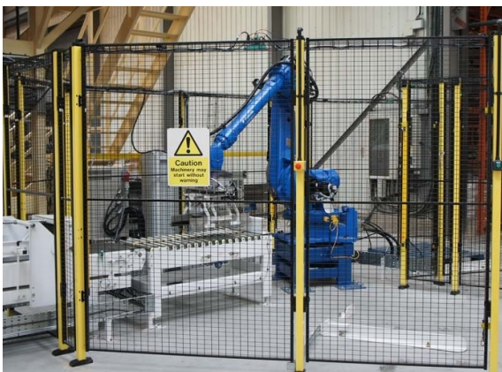
(a) Traditional industrial robot in closed environment, delimited by safety fences and signs prohibiting access to any human individual during robot operation.
