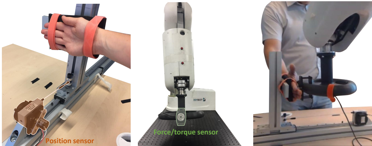
Figure 5.8: Pictures of the test bench: hand of a participant attached to the sliding carriage of the rail ( left ), force/torque sensor located on the steering wheel of the robot ( middle ), human-robot contact with the force/torque sensor at the interface ( right ).
