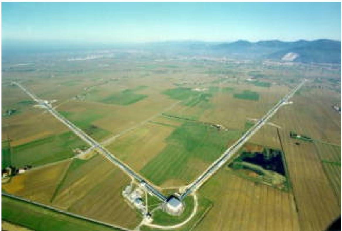
Figure 2.8: A view of the gravitational wave detector, Virgo, from the air. Located in Cascina, Italy, outside of Pisa, the magnitude of the experiment is apparent with its 3 km interferometer arms.
