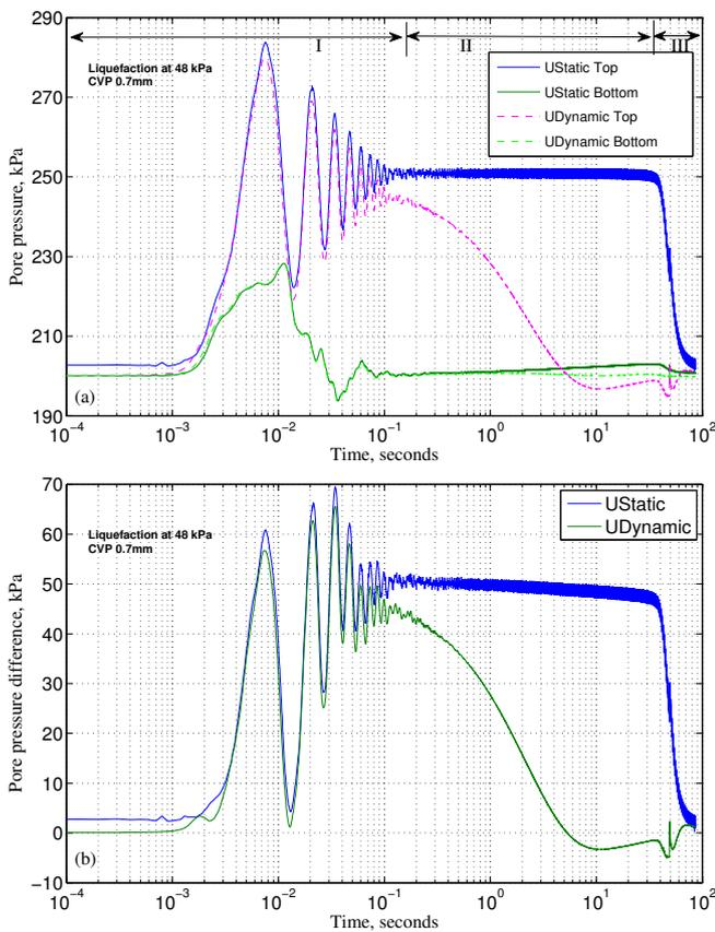
**Fig. 11** (a) Temporal evolution of top and bottom dynamic and static pore pressures, (b) pore pressure difference between top and bottom of isotropic liquefaction at 48 kPa of confining pressure on 0.7 mm CVP beads.
