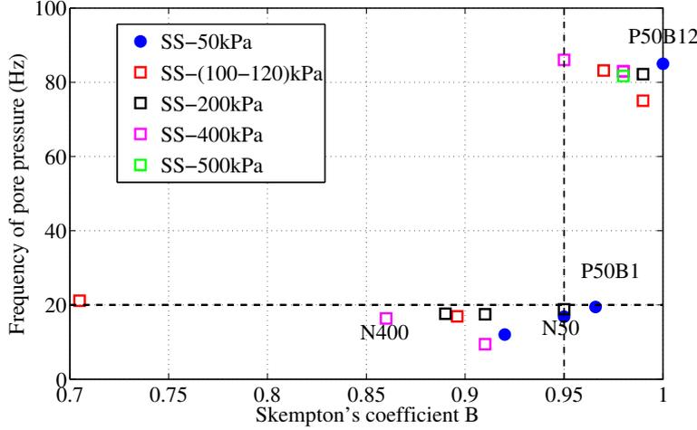
**Figure 4.14:** Variation of frequency of pore pressure in relevance to Skempton's coefficient B.
