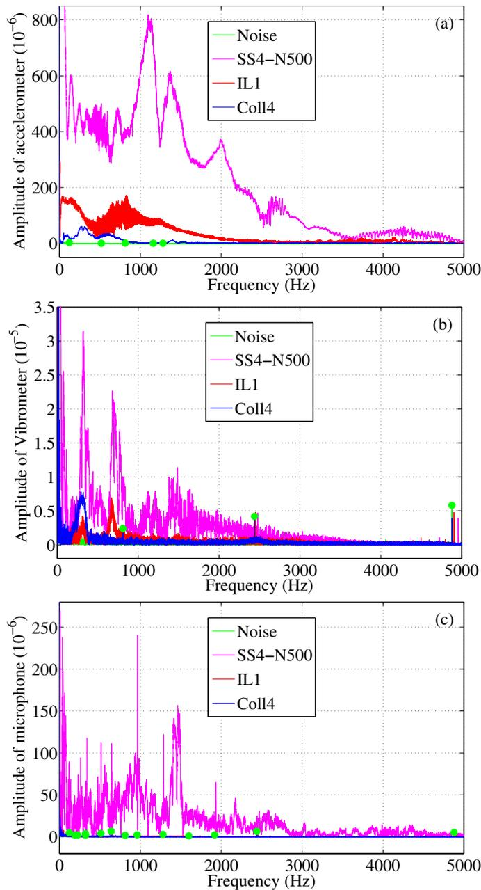
**Figure 6.27:** FFT spectra of collapse Coll<sub>04</sub>, liquefaction IL<sub>01</sub>, stick-slip SS<sub>04</sub>-test N500.
