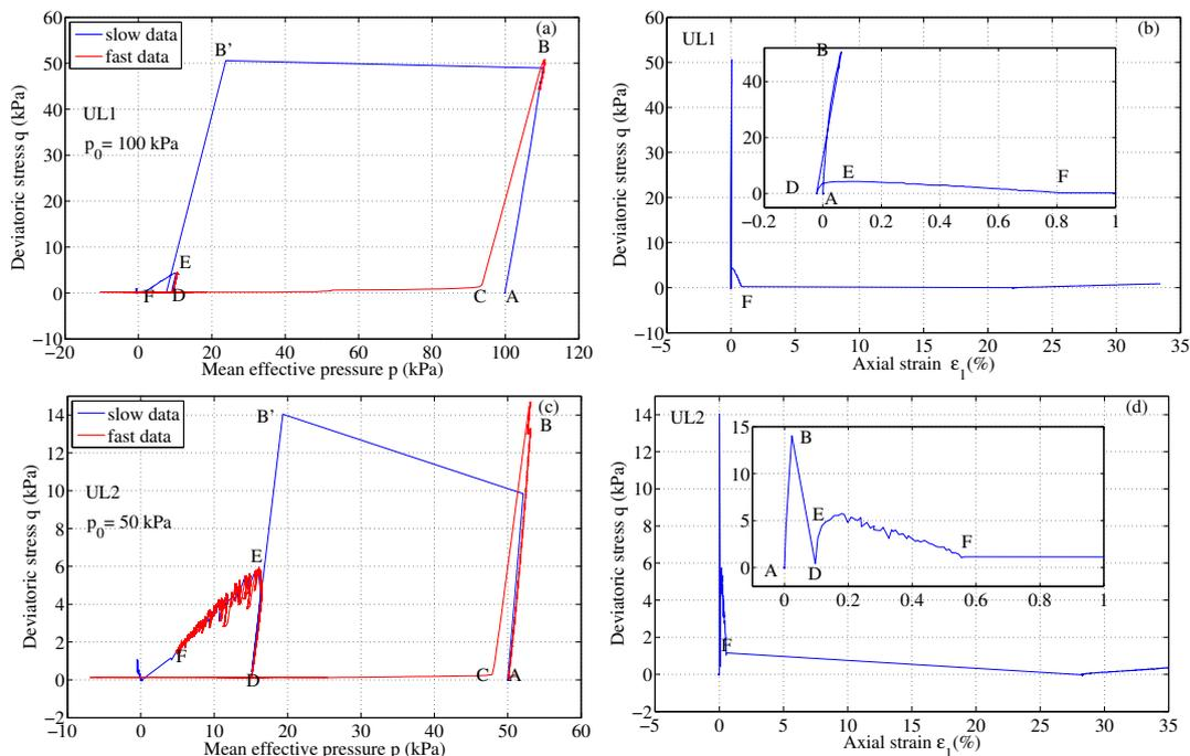
**Figure 5.5:** Global behaviour in static liquefaction of test UL<sub>01</sub> (a,b) and UL<sub>02</sub> (c,d).
