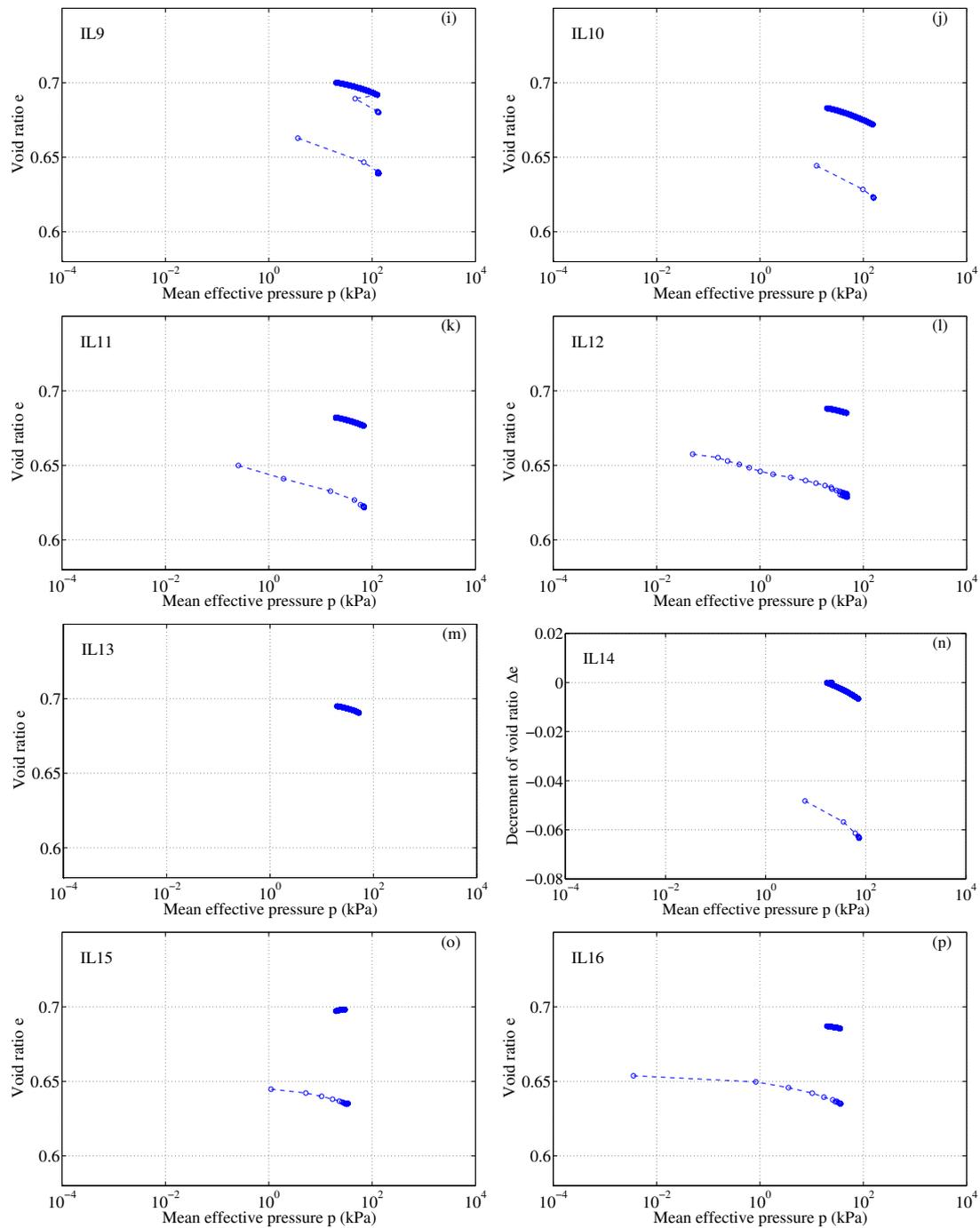
**Figure 5.2:** Compressibility behaviour in isotropic liquefaction (cont, from test IL<sub>09</sub> to IL<sub>16</sub>).
