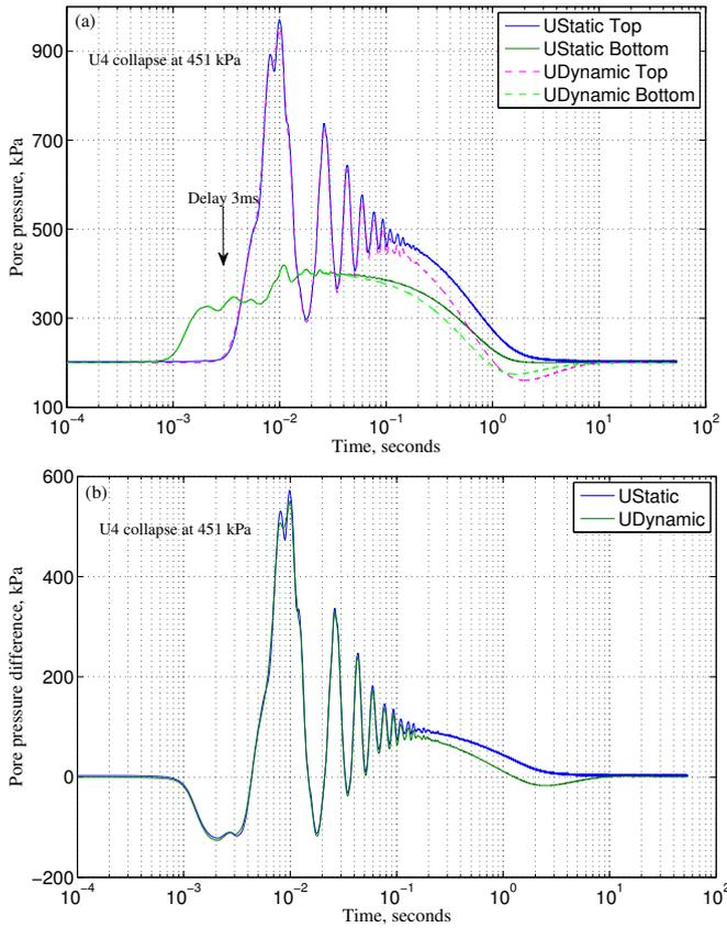
**Fig. 4** (a) Temporal evolution of dynamic and static pore pressures at sample top and bottom. (b) dynamic and static pore pressure difference between top and bottom of isotropic collapse D at 451 kPa of confining pressure on 0.7 mm CVP beads.
