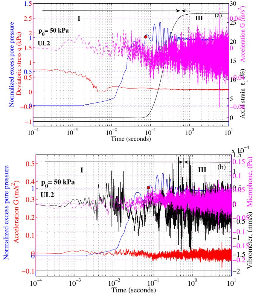
**Figure 5.12:** Detailed behaviour in static liquefaction event UL<sub>02</sub> at initial confining pressure of 50 kPa.
