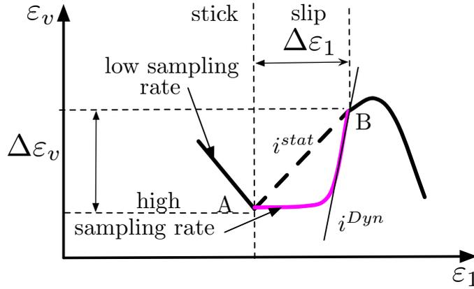
**Figure 4.28:** Static and dynamic anisotropy coefficients for instability.
