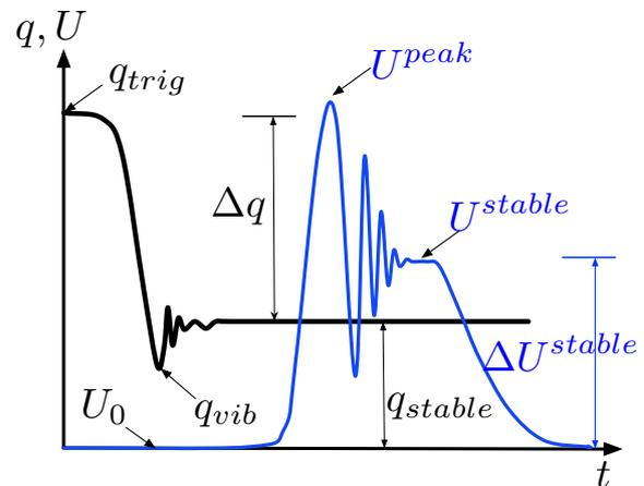
**Fig. 2** Schematic view of the temporal evolution of deviatoric stress  $q$  and pore pressure  $U$  during laboratory dynamic instabilities.
