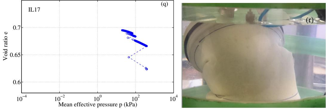
**Figure 5.2:** Compressibility behaviour in isotropic liquefaction (cont, test IL<sub>17</sub>).
