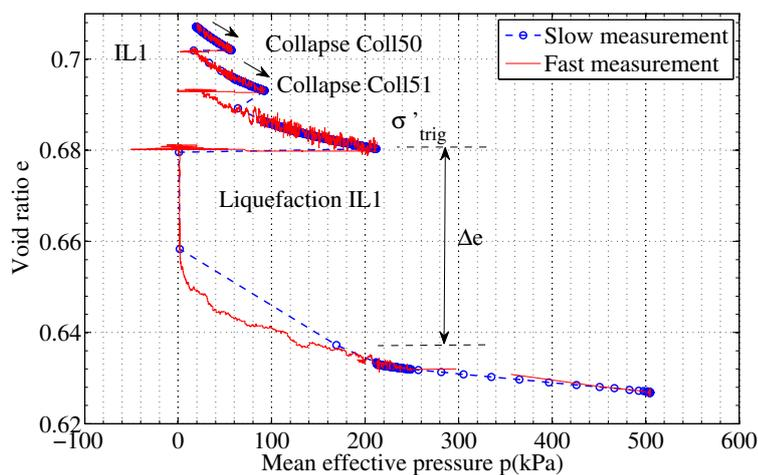
Figure C.2: Compressibility of isotropic liquefaction  $IL_{01}$ .
