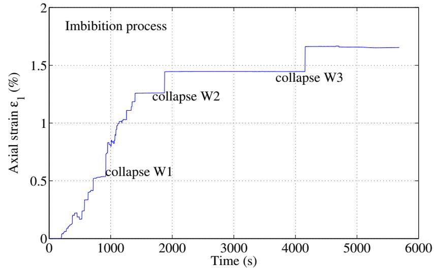
**Figure A.1:** Temporal evolution of axial strain during imbibition process.
