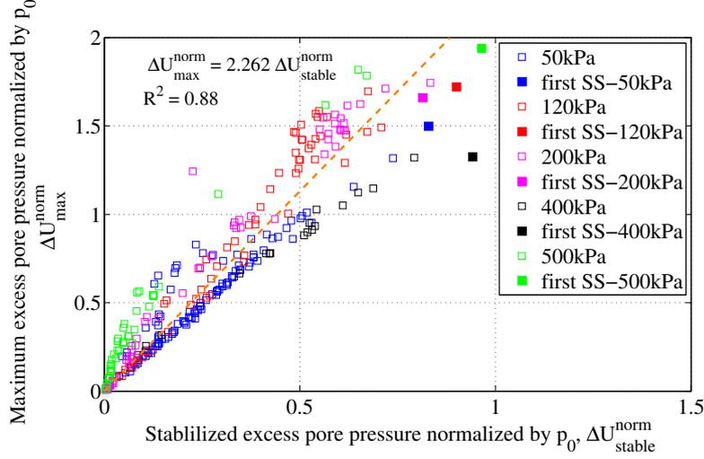
**Figure 4.15:** Maximum and stabilised excess pore pressure normalised by  $p'_0$  in a linear relation.
