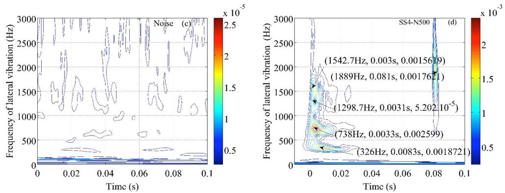
**Figure D.4:** CCWT spectrum of lateral vibration V for noise signal (left) and stick-slip SS<sub>04</sub> of test N500 (right).
