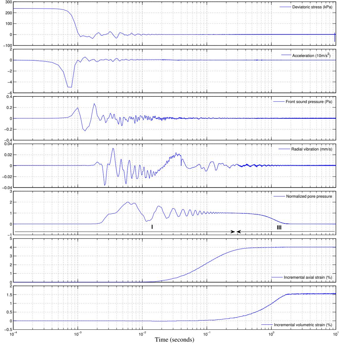
**Figure 4.5:** Temporal evolution inside a typical stick-slip  $SS_{01}$  at 500 kPa (test N500) : Deviatoric stress  $q$ , vertical top cap acceleration, lateral sound pressure, lateral vibration, normalised pore pressure  $U^{norm}$ , incremental axial strain  $\Delta\varepsilon_1$ , incremental volumetric strain  $\Delta\varepsilon_{vol}$ .
