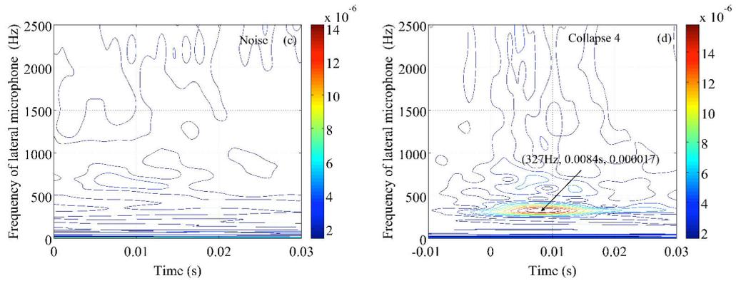
**Figure D.10:** CCWT spectrum of lateral sound pressure M for noise signal (left) and Coll<sub>04</sub> of Collapse series (right).
