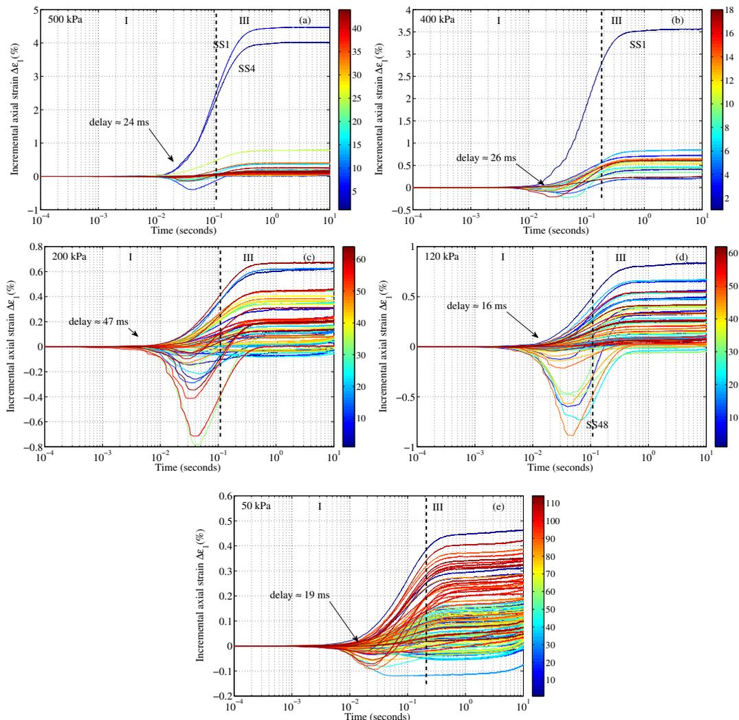
**Figure 4.8:** Time evolution of incremental axial strain  $\Delta\varepsilon_1$  during stick-slip events at (a) 500 kPa of confining pressure, (b) 400 kPa, (c) 200 kPa, (d) 120 kPa and (e) 50 kPa.
