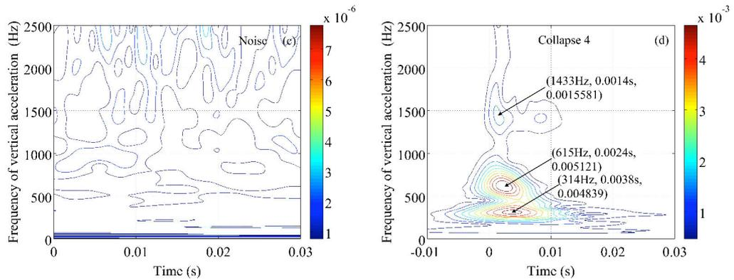
**Figure D.11:** CCWT spectrum of vertical top cap acceleration G for noise signal (left) and Coll<sub>04</sub> of Collapse series (right).
