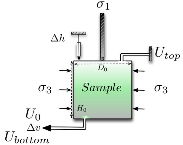
**Fig. 1** Schematic view of the experimental setup for isotropic consolidation and drained triaxial compression.
