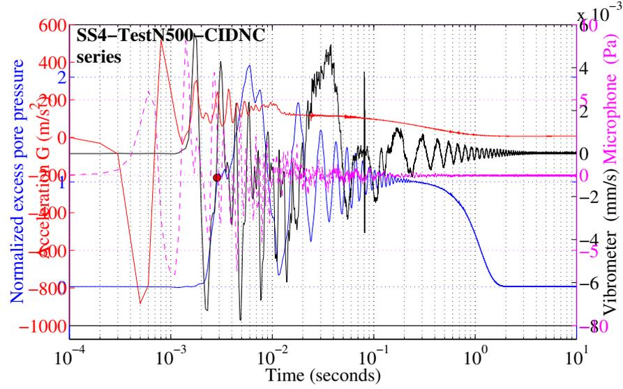
**Figure D.3:** Temporal evolution of acoustic measurements (G,M,V) and normalised excess pore pressure  $\Delta U^{norm}$  during SS<sub>04</sub> of test N500-CIDNC series.
