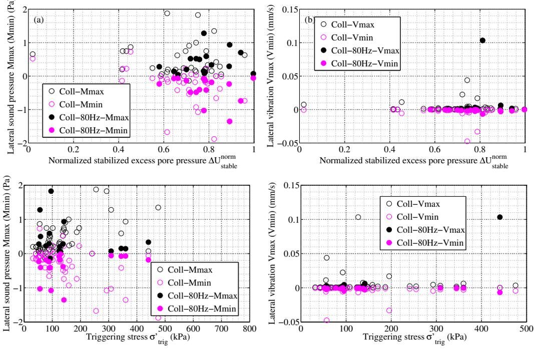
**Figure 6.21:** Relation of amplitude between lateral sound pressure M, lateral vibration V and normalised stabilised excess pore pressure  $\Delta U_{stable}^{norm}$  during collapse events (respectively in accordance with triggering stress  $\sigma'_{trig}$ ).
