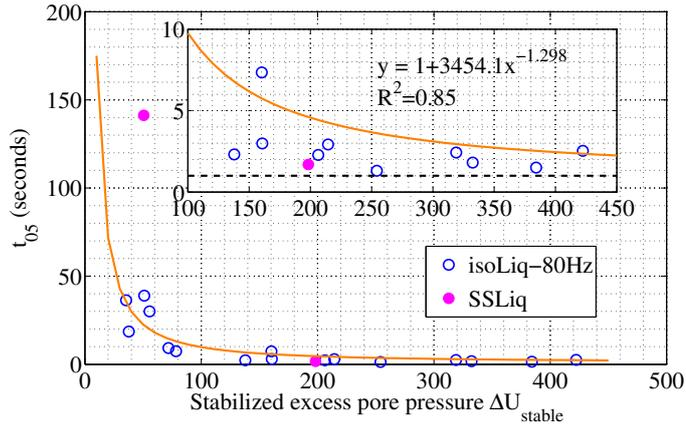
**Figure 5.29:** Evolution of the stabilised phase according to  $\Delta U_{stable}$  during isotropic liquefaction events.
