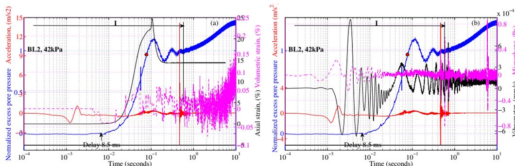
Figure 5.14: Detailed behaviour in liquefaction event BL<sub>02</sub> at effective confining pressure of 42 kPa during application of back pressure.
