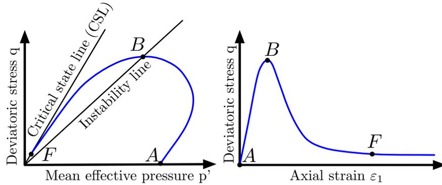
**Figure 5.4:** Static liquefaction of soil in the literature.
