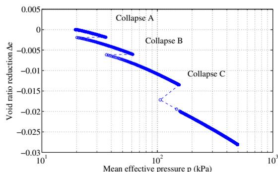
**Figure 5.23:** Compressibility behaviour during isotropic consolidation of slender sample  $H/D = 2$ .
