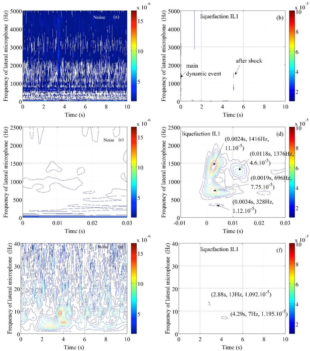
**Figure 6.15:** CCWT spectrum of lateral sound pressure M for noise signal (left) and isotropic liquefaction IL<sub>01</sub> (right).
