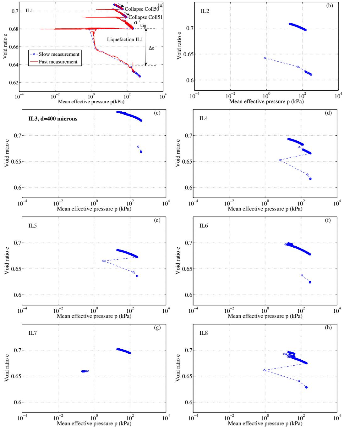
Figure 5.2: Compressibility behaviour in isotropic liquefaction from Test IL<sub>01</sub> to IL<sub>08</sub>.
