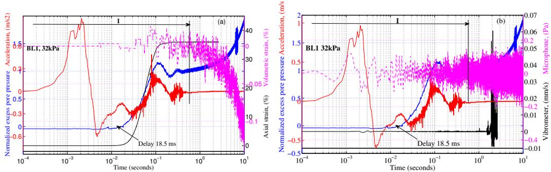
**Figure 5.15:** Detailed behaviour in liquefaction event BL<sub>01</sub> at effective confining pressure of 32 kPa during application of back pressure.
