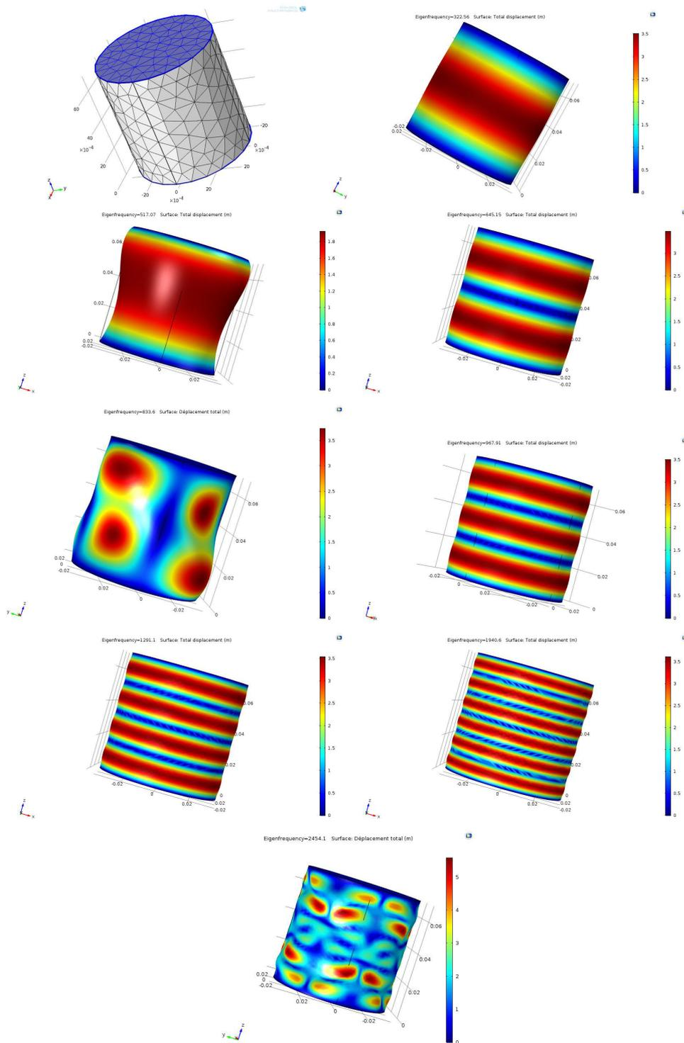
**Figure 6.25:** Model of cylinder saturated granular sample and possible vibration modes at 322, 517, 654, 833, 968, 1291, 1940, 2454 Hz.
