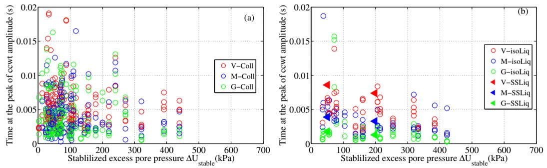
**Figure 6.31:** Time at the peak of CCWT amplitude of collapse (a) and liquefaction (b).
