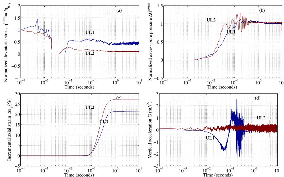
Figure 5.13: Detailed behaviour in static liquefaction events.
