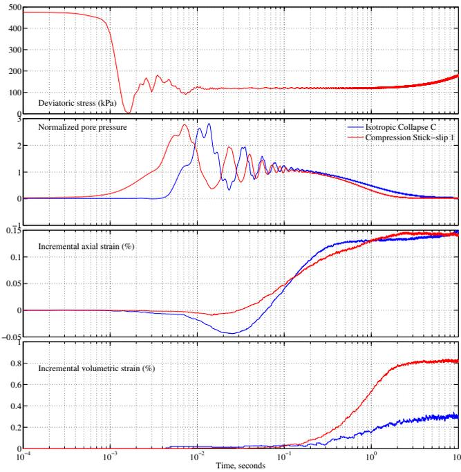
**Fig. 8** Typical temporal evolution of isotropic collapse C (blue) and drained compression stick-slip SS1 (red) on 0.7 mm CVP beads : deviatoric stress, normalised excess pore pressure, axial and volumetric strain.
