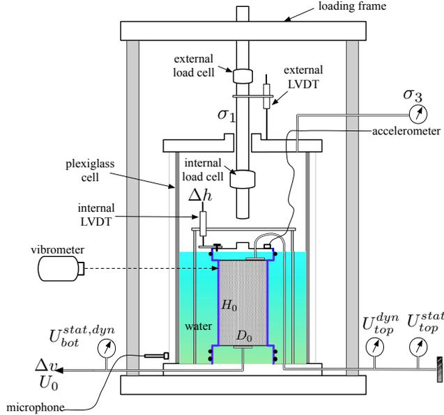
**Figure 3.3:** Scheme of the triaxial test apparatus
