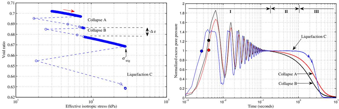
**Figure 2.12:** (left) Spontaneous instabilities under drained isotropic compression, (right) Time evolution of normalised pore pressure during isotropic collapse and isotropic liquefaction (31).
