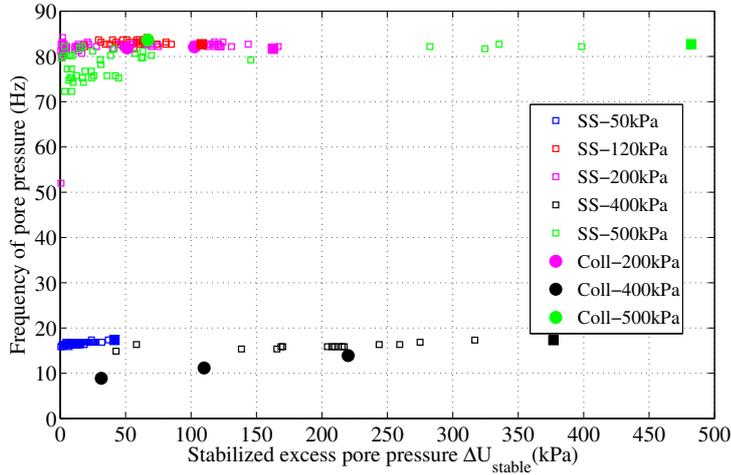
**Figure 4.13:** Effect of stabilised excess pore pressure  $\Delta U_{stable}$  on the frequency of pore pressure.
