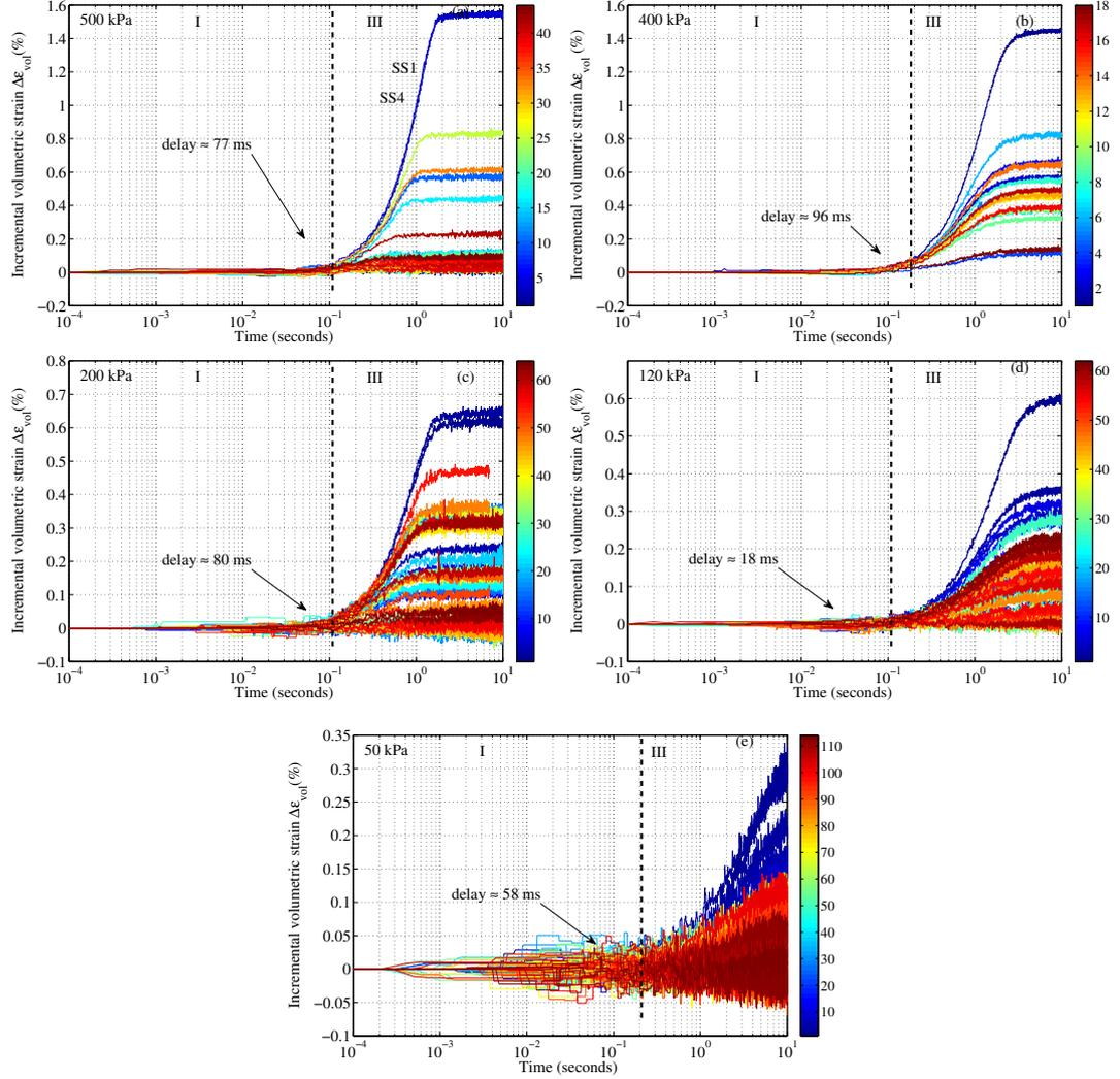
**Figure 4.9:** Time evolution of incremental axial strain  $\Delta\varepsilon_{vol}$  during stick-slip events at (a) 500 kPa of confining pressure, (b) 400 kPa, (c) 200 kPa, (d) 120 kPa and (e) 50 kPa.
