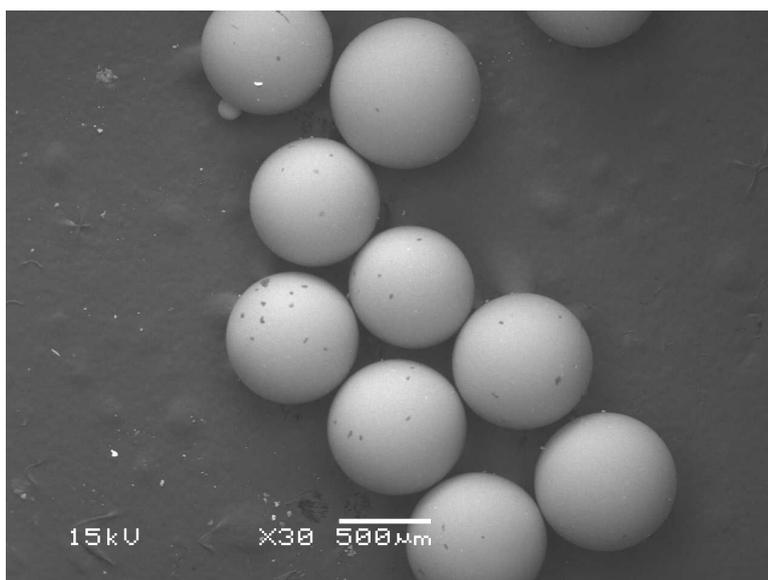
**Figure 3.1:** SEM picture of CVP glass beads
