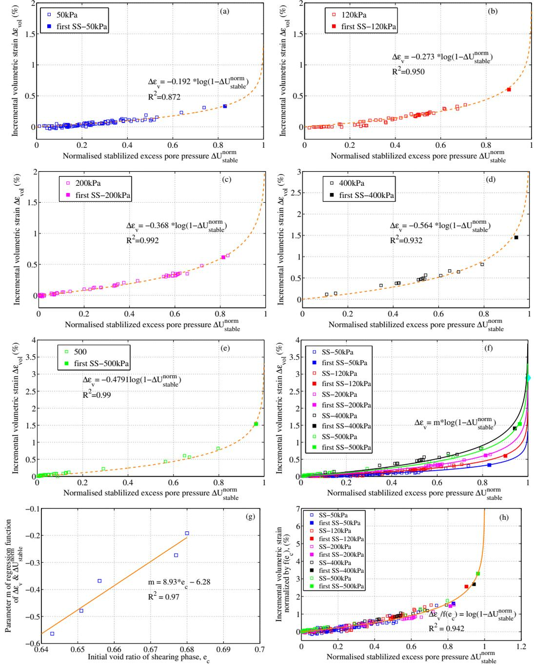
**Figure 4.25:** Normalised stabilised excess pore pressure  $\Delta U_{stable}^{norm}$  and incremental volumetric strain  $\Delta\epsilon_{vol}$  incorporating with the effect void ratio  $e_c$  at the beginning of shearing.
