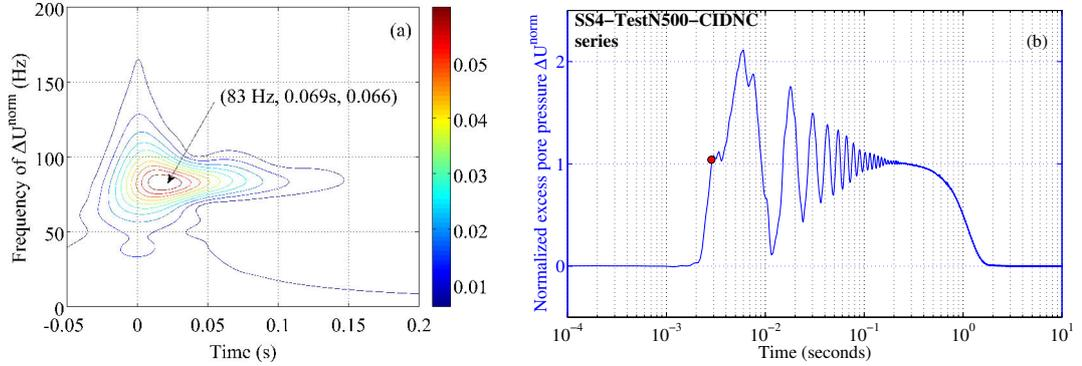
**Figure D.7:** CCWT spectrum of normalised excess pore pressure  $\Delta U^{norm}$  of stick-slip SS<sub>04</sub> of test N500.
