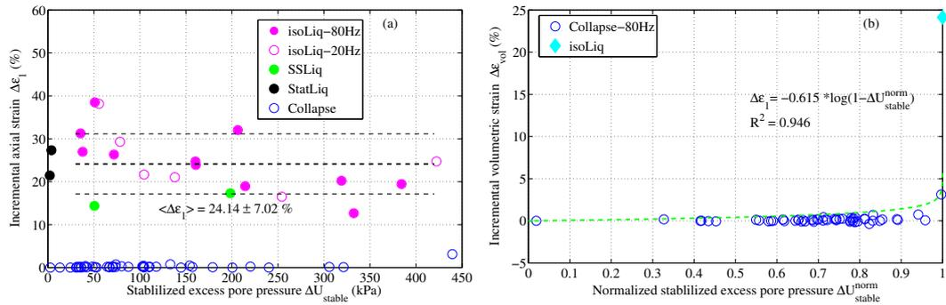
Figure 5.35: Incremental axial strain and stabilised excess pore pressure of liquefaction and collapse.
