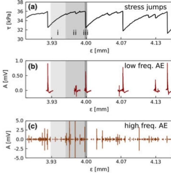
**Figure 2.14:** Stick-slip and acoustic measurements in direct shear stick-slip experiment of 4 mm beads under 60 kPa of confining pressure (81).
