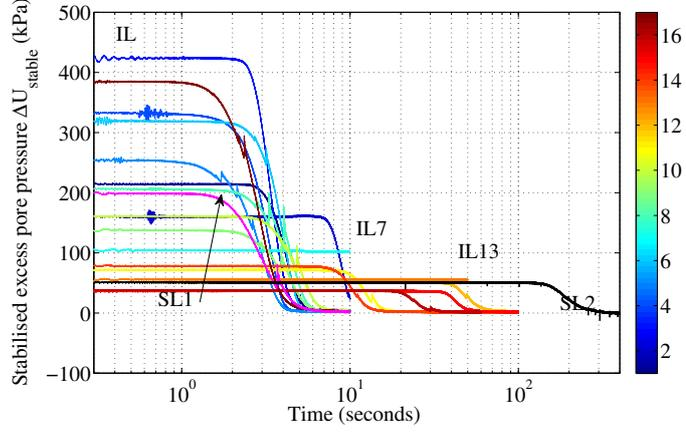
**Figure 5.28:** Dissipation phase of isotropic liquefaction events.
