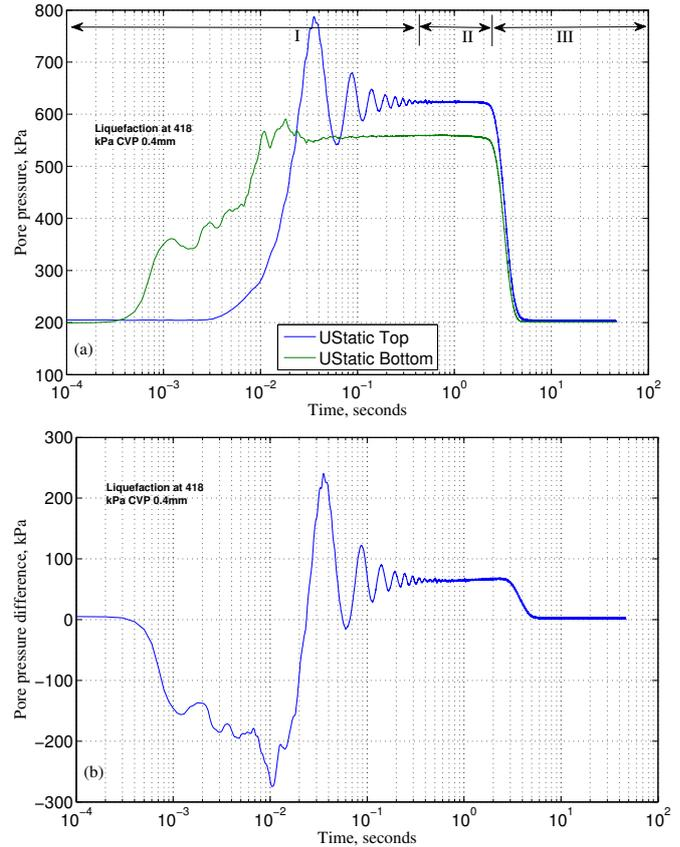
**Fig. 10** (a) Temporal evolution of top and bottom static pore pressures, (b) pore pressure difference between top and bottom of isotropic liquefaction at 418 kPa of confining pressure on 0.4 mm CVP beads.
