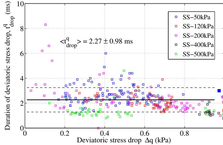
**Figure 4.19:** Duration of deviatoric stress drop  $t_{drop}^q$  in relevance with normalised deviatoric stress drop  $\Delta q^{norm}$ .
