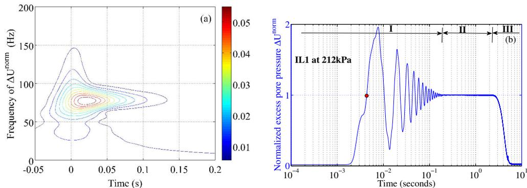
**Figure 6.18:** CCWT spectrum of normalised excess pore pressure  $\Delta U^{norm}$  during isotropic liquefaction  $IL_{01}$ .
