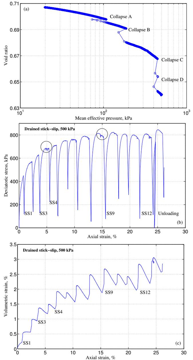
**Fig. 3** (a) Isotropic instabilities from 20 to 500 kPa and (b) drained compression stick-slips with (c) coupled volumetric behaviour at 500 kPa of confining pressure on SLG 6-8 glass beads of 0.7 mm of diameter.
