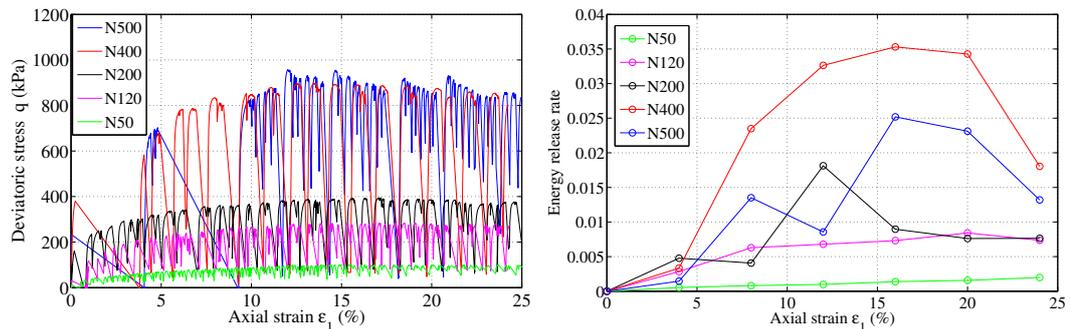
**Figure 6.33:** Energy release rate during shearing stage at different confining pressure (CIDNC series).
