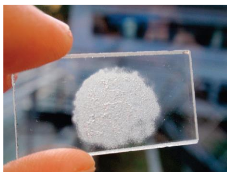
Figure I-10 Erosion of fused silica glass sonicated 180 min in distilled water at 25 °C by 20 kHz ultrasound at 49 \text{ W.cm}^{-2} . [32]
