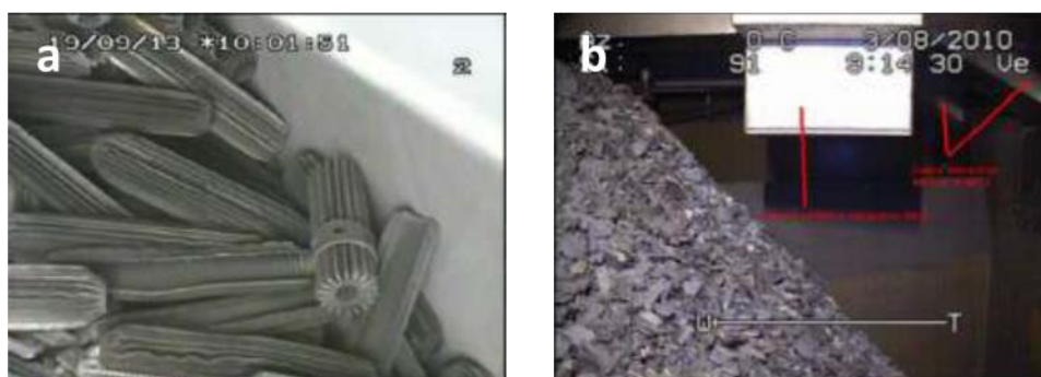
Figure I-22 Mg structural waste stored in wet silos at Marcoule: a) Entire Mg alloy claddings; b) sheared fragments. [1]
