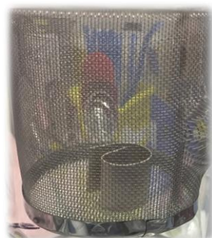
Figure II-5 Tea mesh filter used for samples with a complex geometry.
