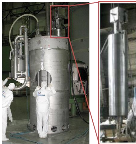
Figure I-27 Ultrasonic cleaning equipment for VVER fuel assemblies in Russia. [169]
