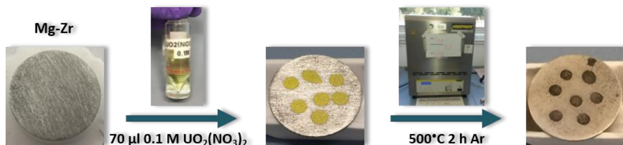
Figure II-2 Mg-Zr disc contamination procedure.
