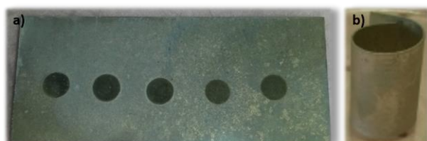
Figure II-3 Mg ribbon contaminated with a 0.1 M \text{UO}_2(\text{NO}_3)_2 aqueous solution a) after heating, b) bent in the form of a cylinder to simulate a sample with a complex geometry.
