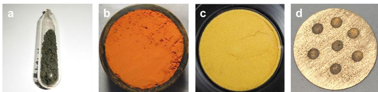
Figure V-7 Photos of: a) U_3O_8 produced by heating ammonium diuranate; [254] b) \beta - UO_3 powder; c) \gamma - UO_3 powder [255] and d) as-prepared contaminated Mg-Zr surface ( 0.1\text{ M } UO_2(NO_3)_2 ).
