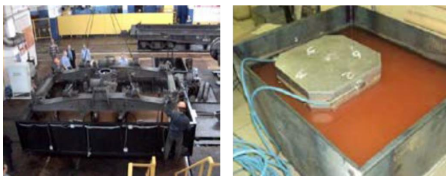
Figure I-29 MO-21 ultrasonic bath (left) and a remotely controlled ultrasonic module (right). [169]
