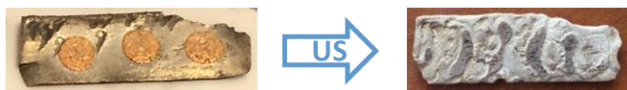
Figure V-15 Photos of an as-prepared contaminated UNGG cladding fin side sample (0.1 M \text{UO}_2(\text{NO}_3)_2 ) before and after 345 kHz sonication ( P_{ac}= 40 W) during 90 min in 0.01 M oxalic acid, Ar, stirring 100 rpm, 20 °C.
