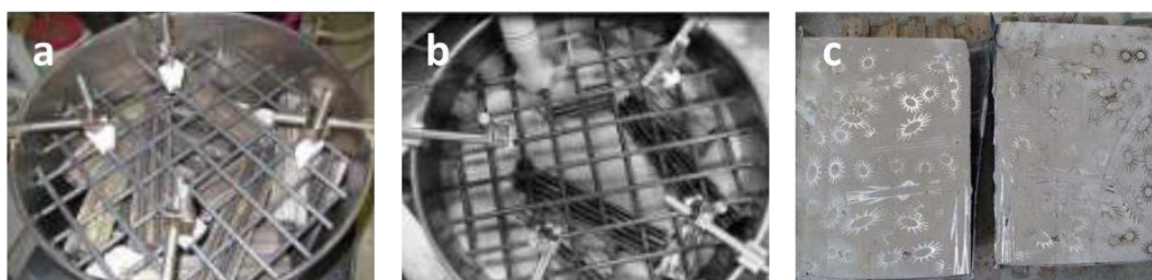
Figure I-23 Inactive simulated Mg claddings in 223 L stainless steel container: a) before grouting; b) geopolymer material grouting; c) profile view after cutting the grouted package. [1]
