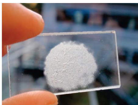
Figure I-10 Erosion of fused silica glass sonicated 180 min in distilled water at 25 °C by 20 kHz ultrasound at 49 \text{ W.cm}^{-2} . [32]
