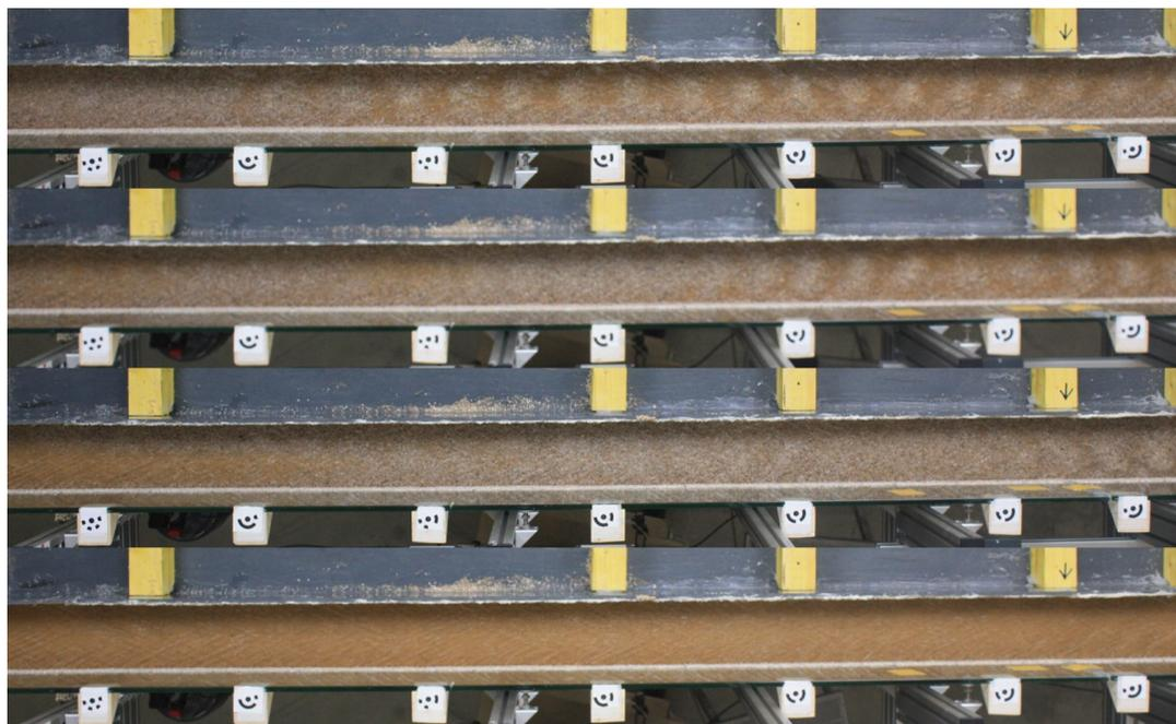
FIGURE 4.27: Run3. Top view of the central part of the flume, flow is from left to right. The time interval between the first photo, at the top of the figure, and the last one, at the bottom of the figure is about 30 minutes. In this half an hour, as well as for all run's duration, photos were taken with a frequency of one per minute.
