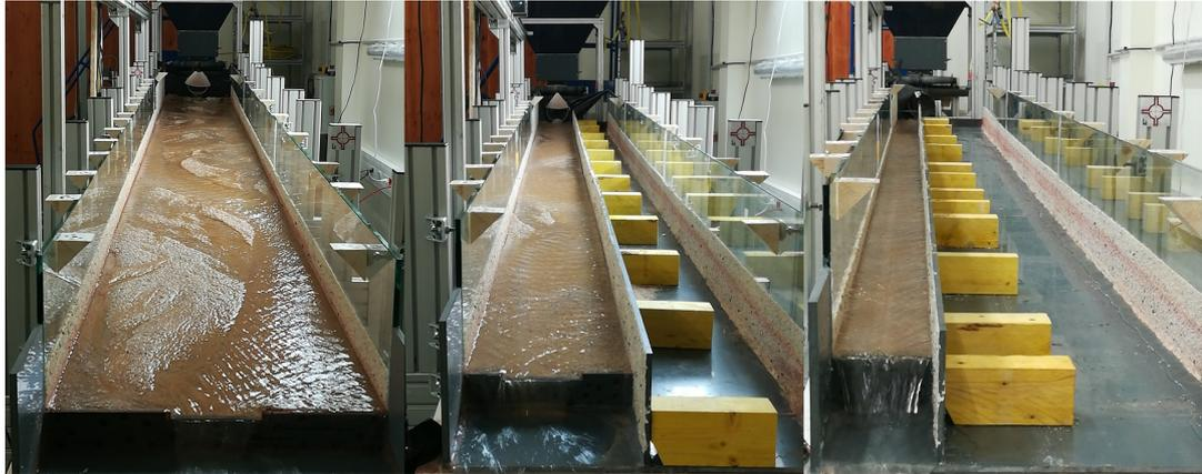
FIGURE 4.9: The three runs configurations. Left figure: Run 1, flume width 0.5 m. Central figure: Run 2, flume width 0.25 m. Right figure: Run 3, flume width 0.12 m.
