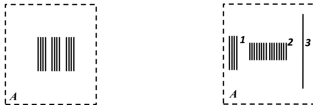
Figure 5.1: A schematic representation of the initial distribution of the micro-cracks. Left: single micro-cracks family model (F1). Right: 3 micro-cracks families model (F3). Note that the two models have the same damage, and the second model has an uniformly distributed damage on all three micro-crack types.
