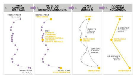
Figure 6.1. Transformation of raw GPS points into trips and Origin-Destination segments.
