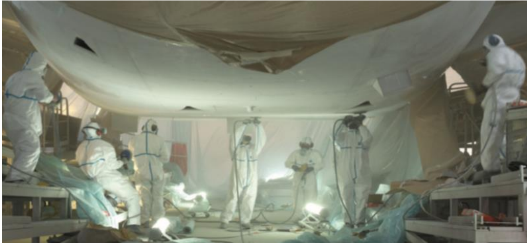
Figure 1.2: Stripping of the bottom part of the airplane manually.
