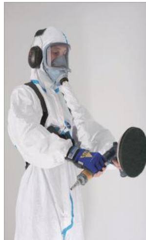
Figure 1.1: Protection for the sanding phase
