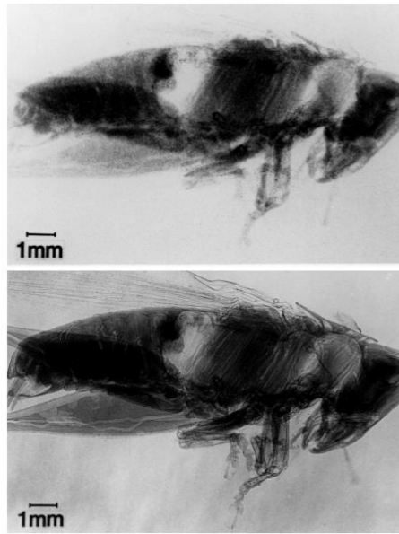
Figure 17: Pure absorption image (above) and phase contrast image (below) of a locust [131] .
