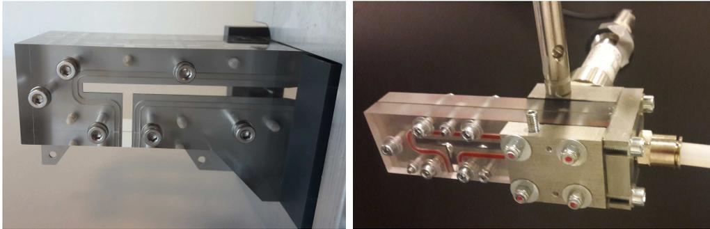
Figure 4.3: The atomizer with acrylic transparent material on the left (Sou et al., 2012), and BK7 glass on the right.
