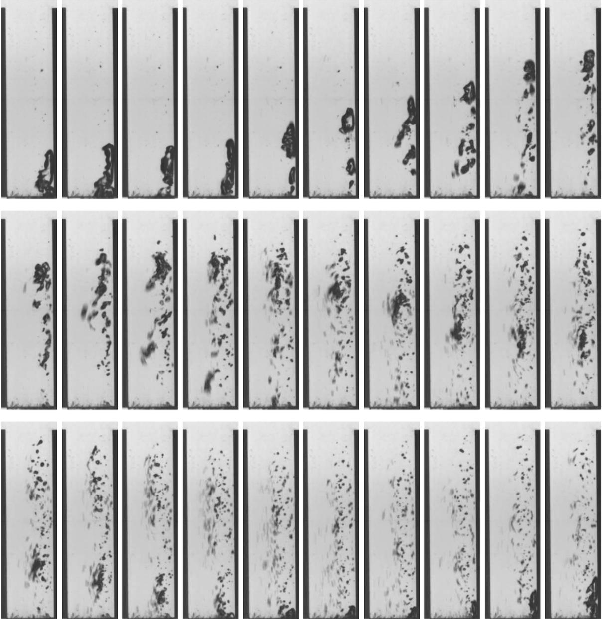
Figure 5.4: Sequence of images of G2-1 from the left to right pictured over 13.92 ms (time delay between images  $480 \mu\text{s}$ ) using the optical system No. II in Table 4.7.
