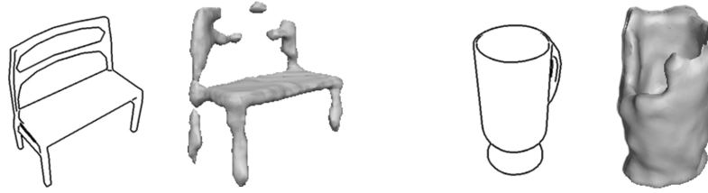
Figure 2.14: Thin structures are challenging to capture by the 64^3 voxel grid.
