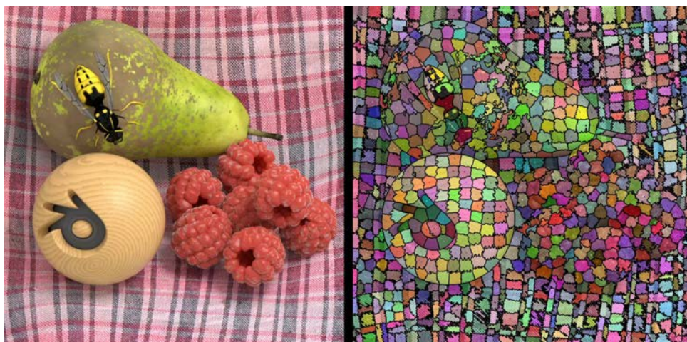
Figure 4: An example of super-rays obtained using the algorithm in [46]. For visualization purpose, the result is shown for only one view of the Light Field StillLife . On the left, the original view in the RGB space. On the right, the resulting super-rays.
