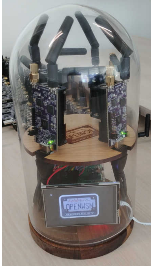
Figure B.1: At OtBox: a Raspberry Pi, 4 OpenMote B boards, a screen and a QR code in a glass dome.
