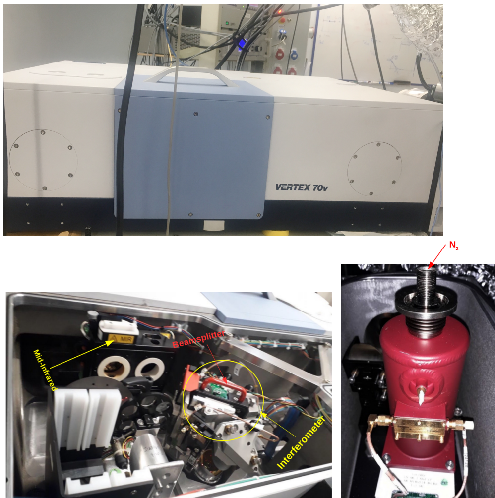
FIGURE 2.5: Photos of the external and internal Vertex 70v (top and left panel) and MCT detector (right panel)
